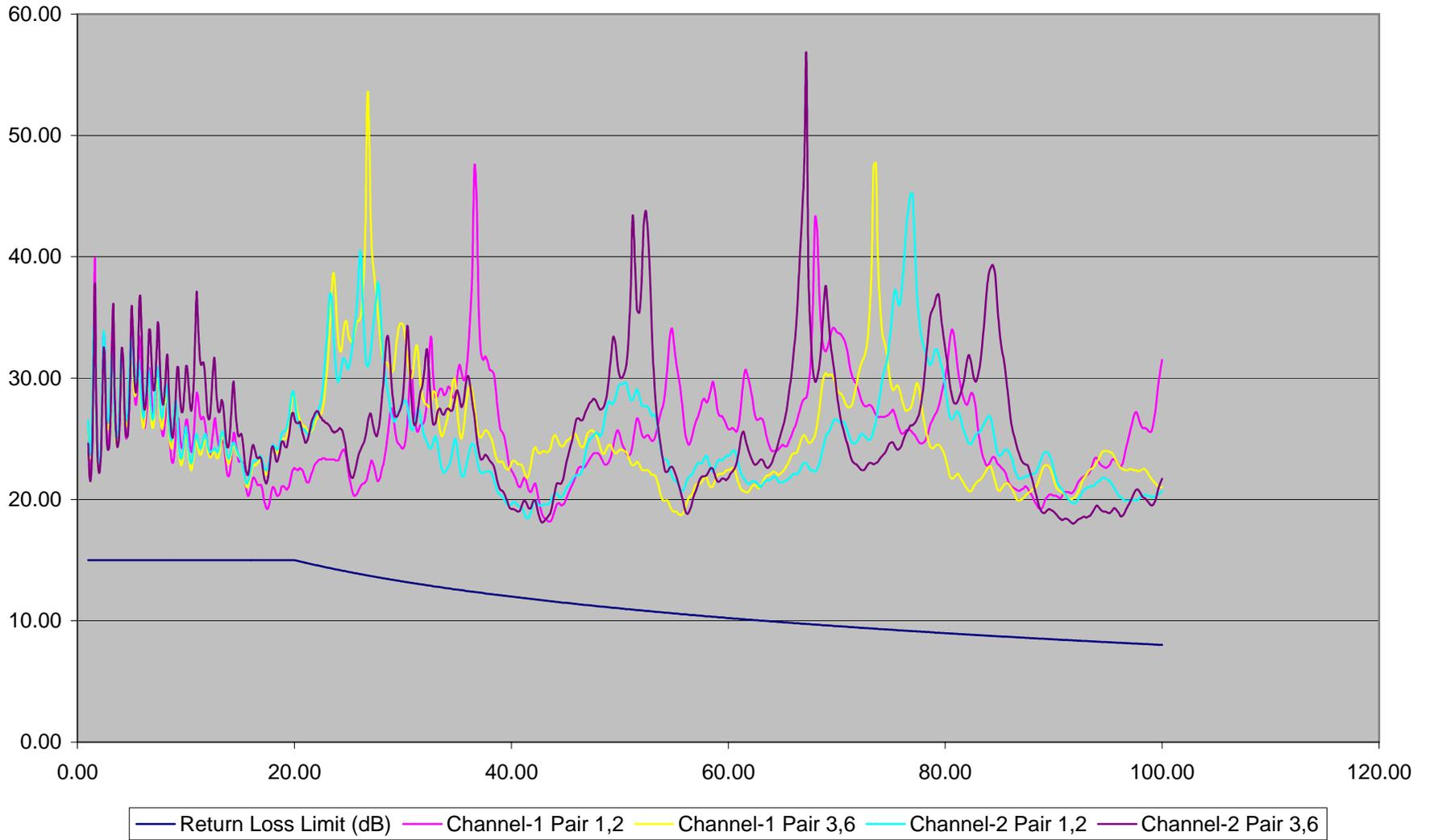
**CAT 5 - TSB95 Spec @ Maximum Attenuation - Return Loss @ Remote**
