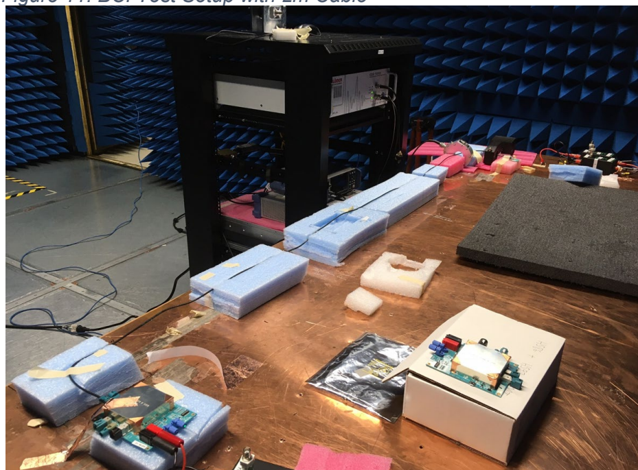
Figure 12. BCI Test Setup with 2m Cable
