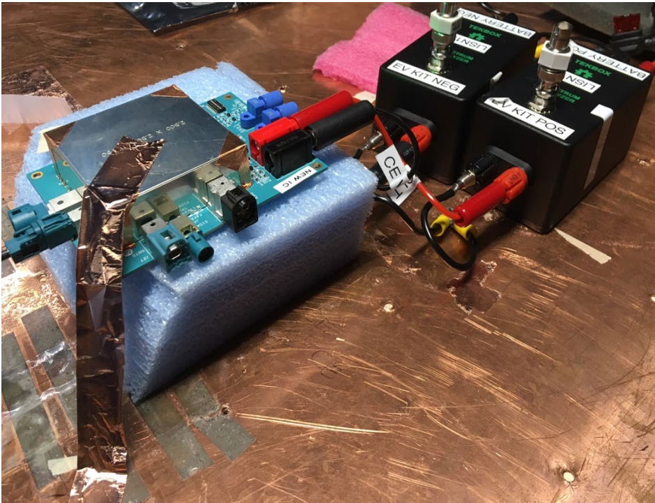
Figure 13. BCI Test Setup with 2m Cable
