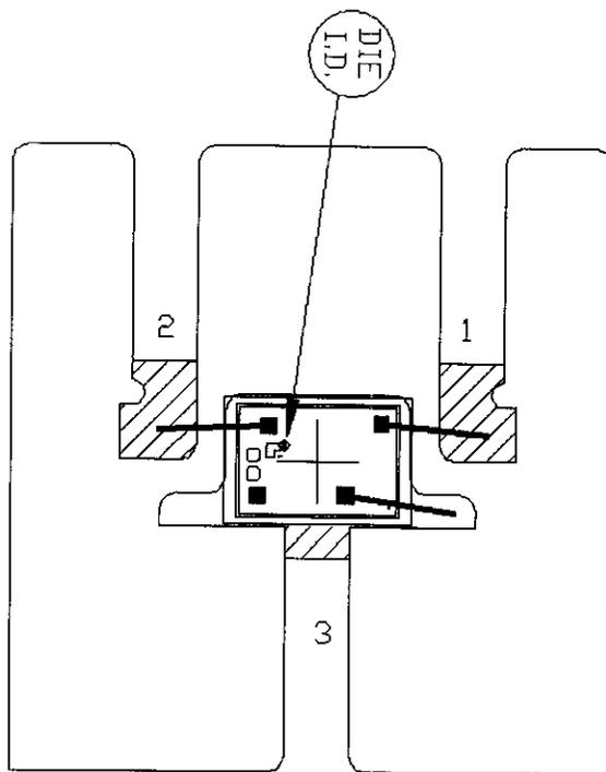
NOTE: USE NON-CONDUCTING EPOXY DIE ATTACH
