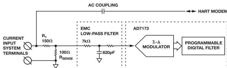
Figure 2. HART enabled, flexible bandwidth input.
