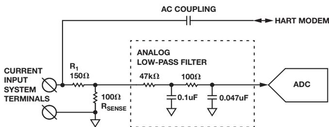
Figure 1. HART enabled input with passive filter.
