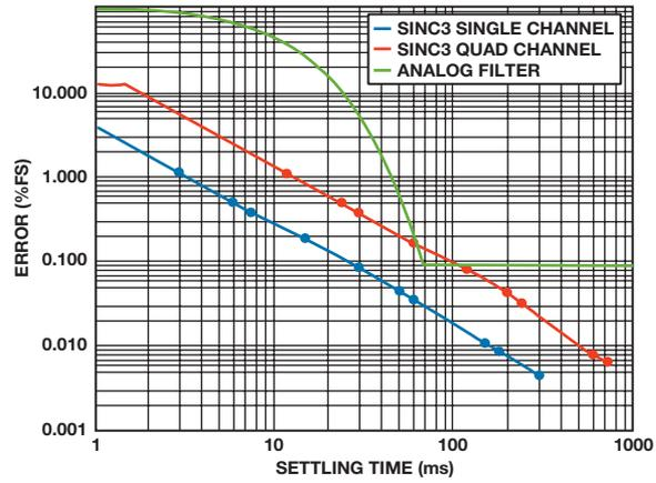
Figure 5. Sinc3 filter vs. analog filter.
