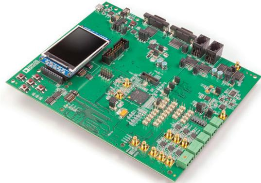
Figure 8. ADSP-CM419F evaluation board.
