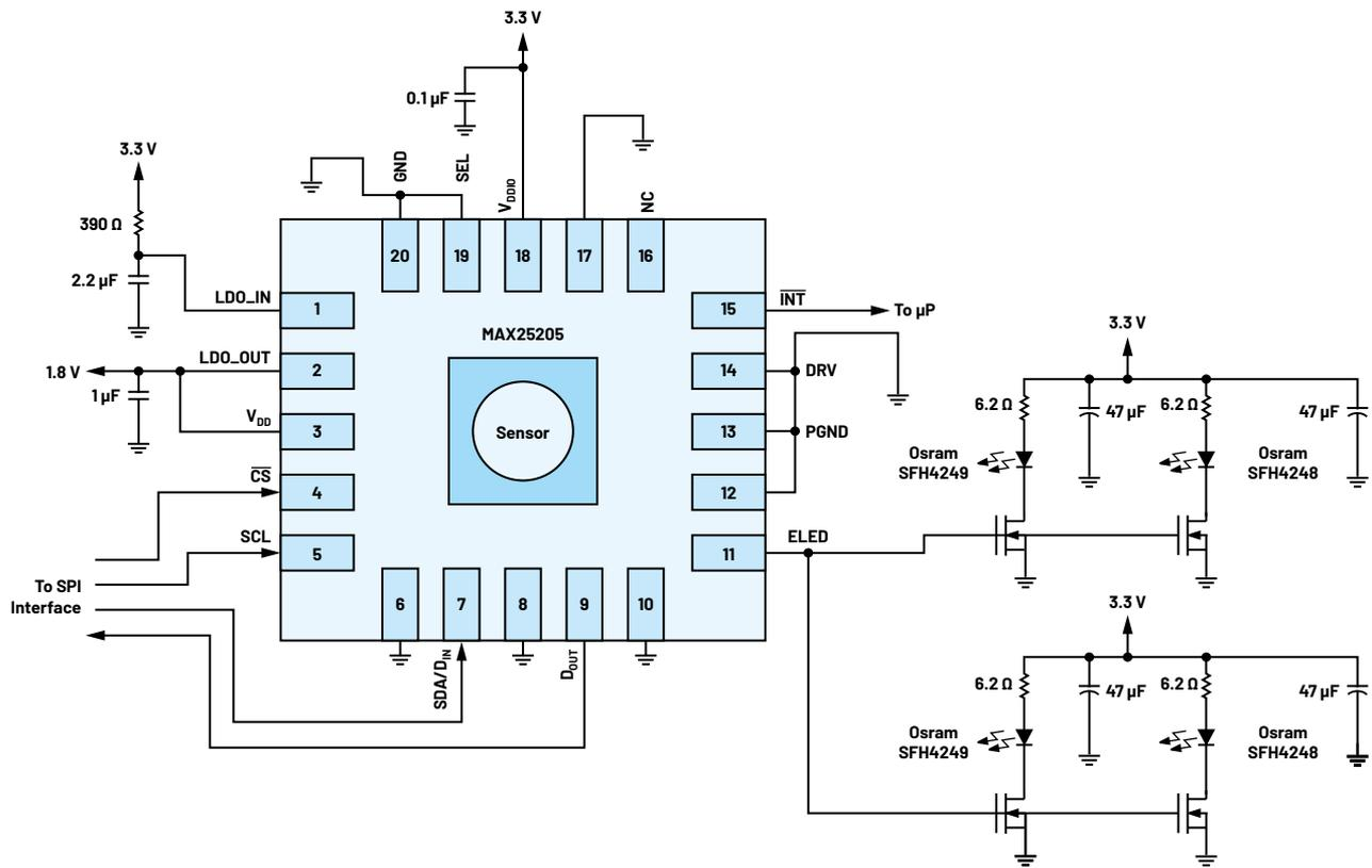
Figure 6. An integrated gesture sensor application diagram.
