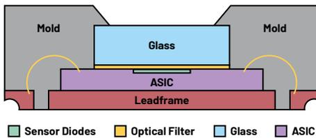
Figure 3. Integrated optics and AFE cross-section.
