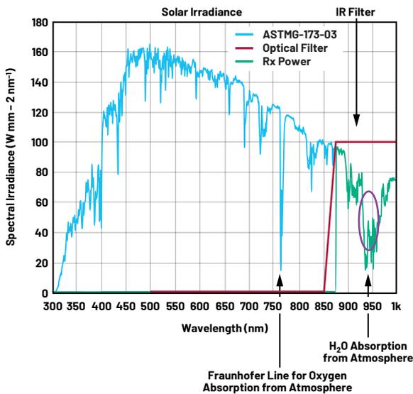
Figure 4. Protecting the sensor from solar irradiance.
