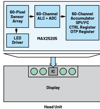
Figure 5. Integrated gesture sensor ensemble.
