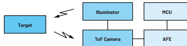
Figure 1. Typical application using a ToF system.
