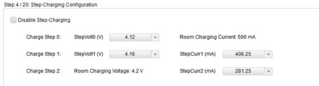
Figure 3. Enable step charging.
