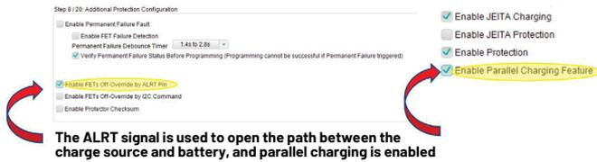
Figure 2. Configuring the MAX17330 for parallel charging.
