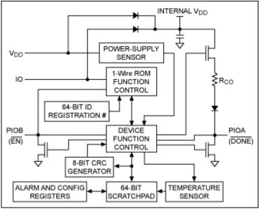
Figure 3. Able to run from either parasitically derived power or from an external supply, the DS28EA00 combines a temperature sensor, GPIO, alarm capabilities, and the 1-Wire interface in an 8-pin micro-small-outline package ( $\mu$ SOP).
