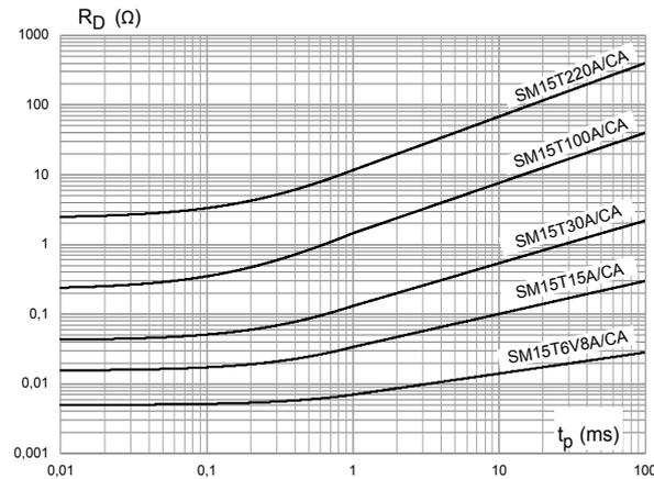
SM15T39A is not plotted on Figure 7. However, we will use the SM15T30A, showing a ratio  $\approx 2$  between  $R_D$  at 1 ms and  $R_D$  at 2 ms.
