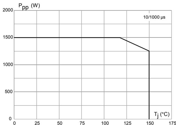
Peak power capability at 150 °C remains at high level:  $P_{PP} = 1250 \text{ W}$  (83% of peak power at 25 °C).
