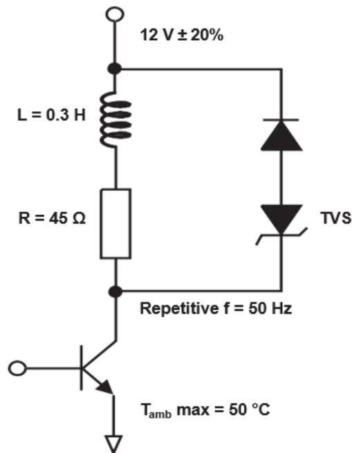
For this usual topology, each time the transistor turns off, a spike (called later  $V_{spike}$ ) is generated due to the inductive effect. This spike reaches very high voltage value and would damage the transistor if no protection is implemented.
