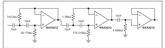
Figure 4. Transposing resistors and capacitors in the Figure 3 circuit yields a 5th-order, 1dB-ripple Chebyshev highpass filter.
