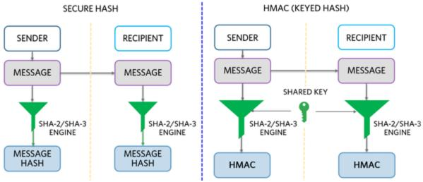
Figure 4. Secure hash and HMAC.
