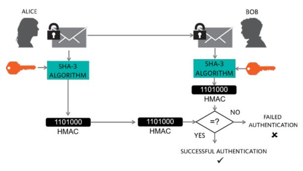
Figure 5. Message authentication using SHA-3 HMAC.
