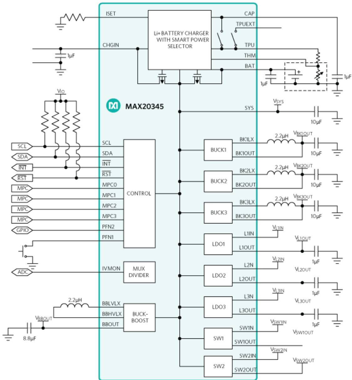
Figure 8. MAX20345 PMIC with a buck-boost converter.
