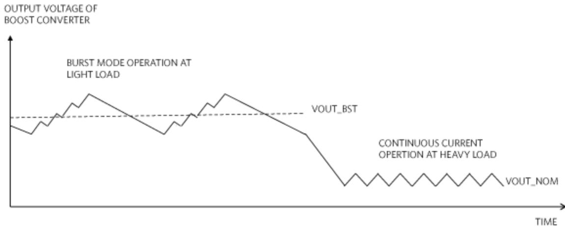
Figure 3. Light and heavy load conditions of a boost converter.
