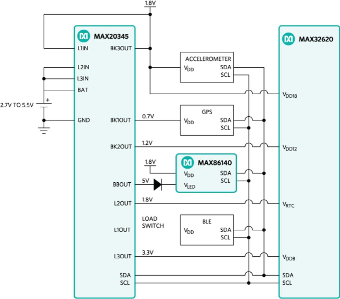
Figure 10. PMIC with buck-boost regulator powers multiple peripherals, sensors, and a microcontroller.
