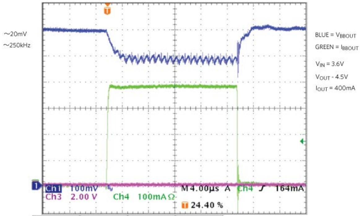
Figure 9. Burst mode ripple of a buck-boost converter with lower amplitude (MAX20345).
