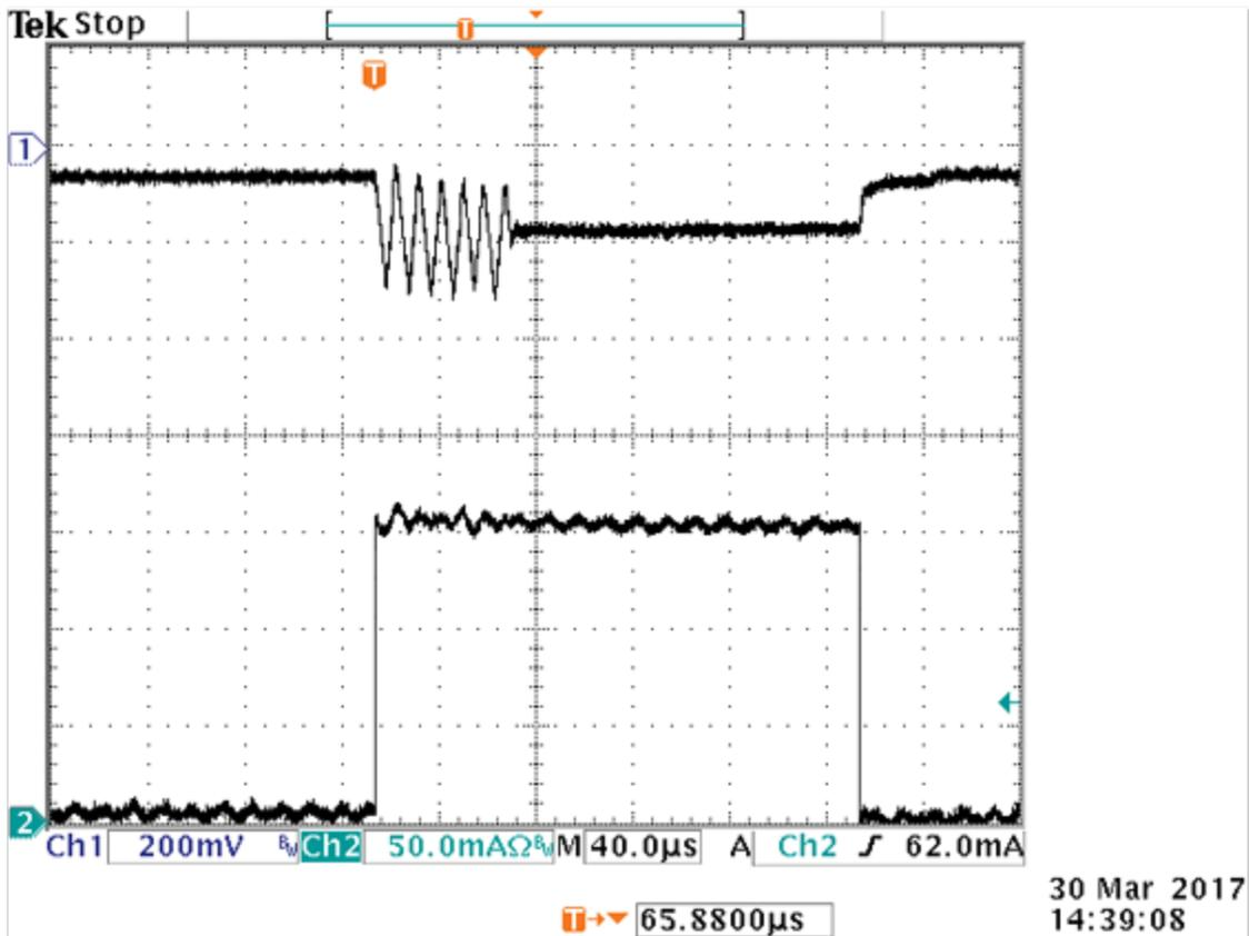
Figure 5. Noise during transition between modes.
