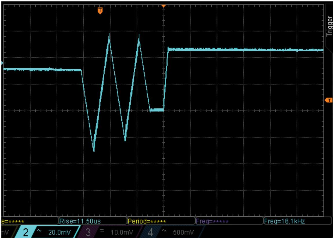
Figure 7. Slow response to load transients of a single-pulse duration.
