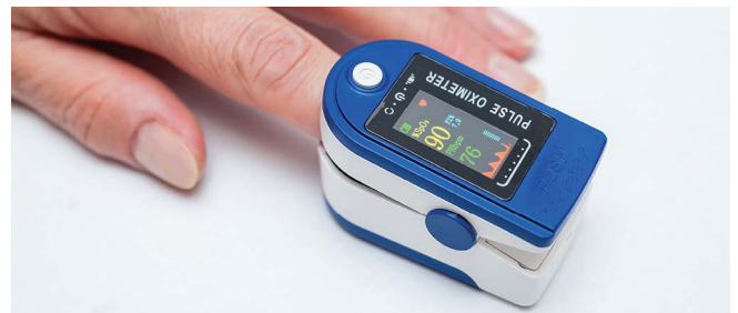
Figure 2. Finger-worn pulse oximeter measuring SpO_2 .
