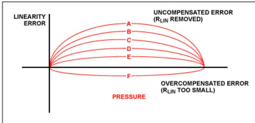
Figure 5. Changing the feedback value ( $R_{LIN}$ ) adjusts the linearity error to the user's specification.
