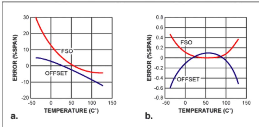
Figure 4. An actual example of uncompensated sensor error demonstrates the difficulty involved in achieving accuracy better than  $\pm 0.1\%$  or even  $\pm 1\%$  (a). Small errors remain after compensating the signal transducer (b).
