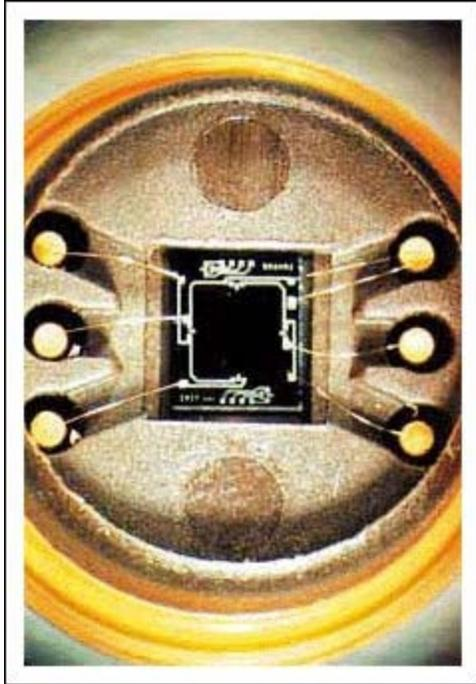
*Photo 3. After anodic bonding to a Pyrex glass wafer, the individual chips are cut out of the wafer, bonded into a package such as the metal can shown here, and wire-bonded to the electrical connectors. Because Pyrex and silicon have virtually identical thermal extension coefficients, thermal tensions are eliminated by the bonding step.*
