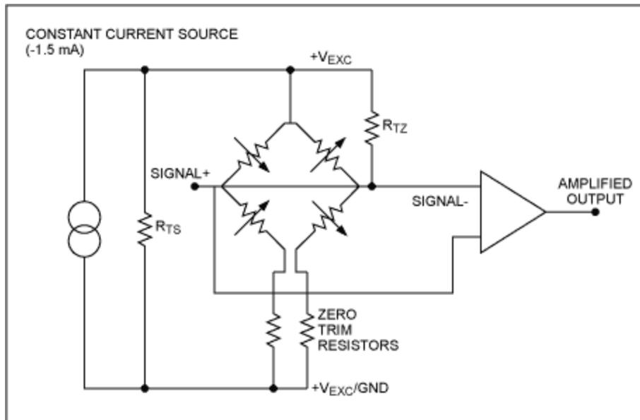
Figure 1. Interaction of the three compensation mechanisms in a conventional resistive compensation circuit ( $R_{TS}$  for sensitivity drift,  $R_{TZ}$  for offset drift, and zero-trim resistors) makes it quite difficult to compensate the overall temperature drift.
