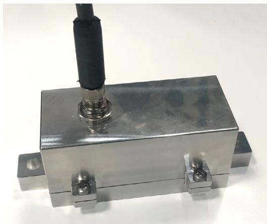
Figure 1. 10BASE-T1L single-pair Ethernet conditioning monitoring (vibration) sensor prototype.
