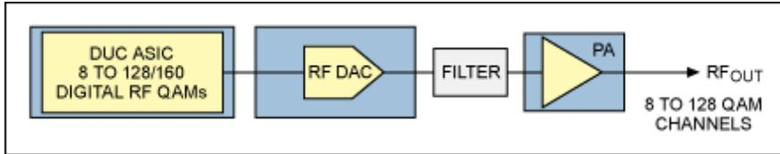
Figure 3. A direct RF transmitter is a single signal chain.
