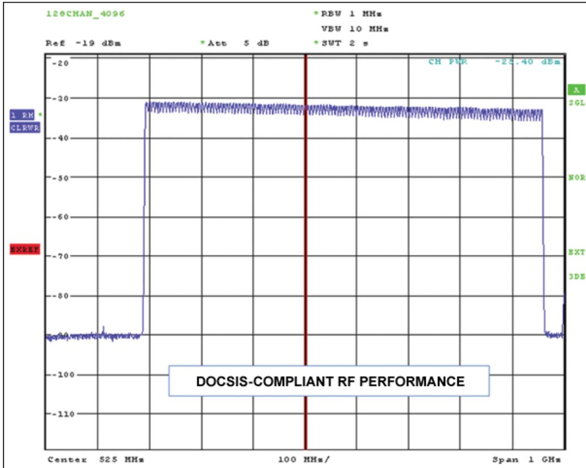
Figure 6. Cable RF spectrum of 128 QAM channels using the DUC (MAX5880) and RF DAC (MAX5882) chipset.
