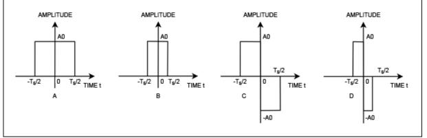
Figure 5. The MAX5879 RF DAC's impulse response for a) NRZ mode; b) RZ mode; c) RF mode; and d) RFZ mode.
