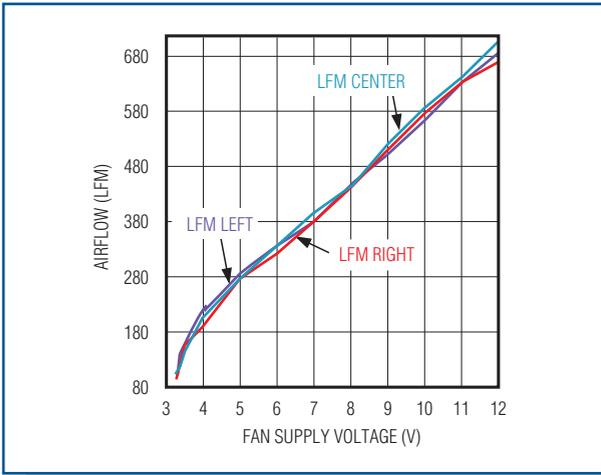
Figure 3a. With the test box empty, three airflow measurements provide baseline information.
