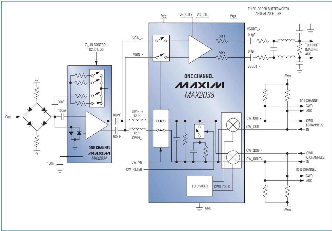
Figure 3. This simplified single-channel ultrasound receiver features the MAX2038 and MAX2034. The MAX2038 integrates eight VGA and CWD I/Q mixer/beamformer channels, and the MAX2034 integrates four LNA channels.
