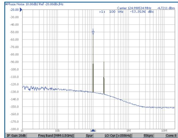
Figure 7. Measured SSB phase noise and spur.
