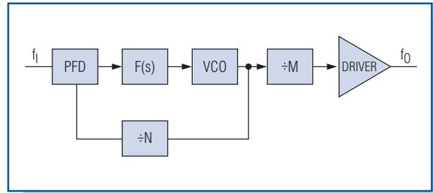
Figure 1. A typical topology for a PLL clock generator.
