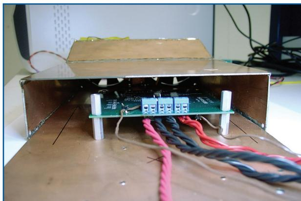
Figure 1. The thermal derating box surrounds the EV board and keeps the airflow predictable to ensure reproducible measurements.
