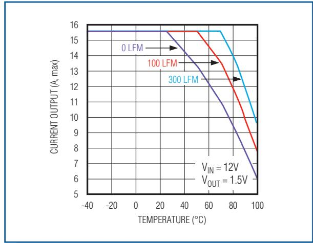
Figure 4a. Maximum output current vs. ambient temperature for the MAX15035. With the MAX15035 EV board in the test box, the thermal derating curves are determined for three different levels of airflow.
