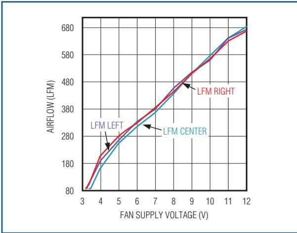
Figure 3b. With the EV board inserted into the test box, the airflow measurements are repeated to identify differences in the airflow vs. the empty box.
