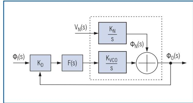
Figure 2. The phase model for a PLL.
