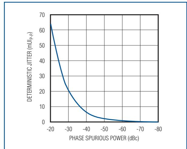
Figure 4. DJ vs. phase spurious power.
