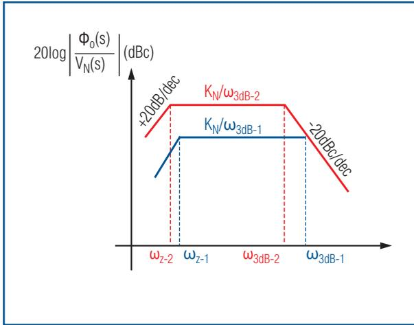
Figure 3. Typical PLL PSNR characteristics.
