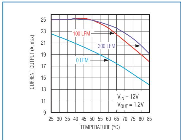
Figure 4b. Maximum output current vs. ambient temperature for the MAX8686. The thermal derating graph of the MAX8686 shows that at +50°C ambient the controller can handle its rated 25A current with as little as 100 LFM of airflow.
