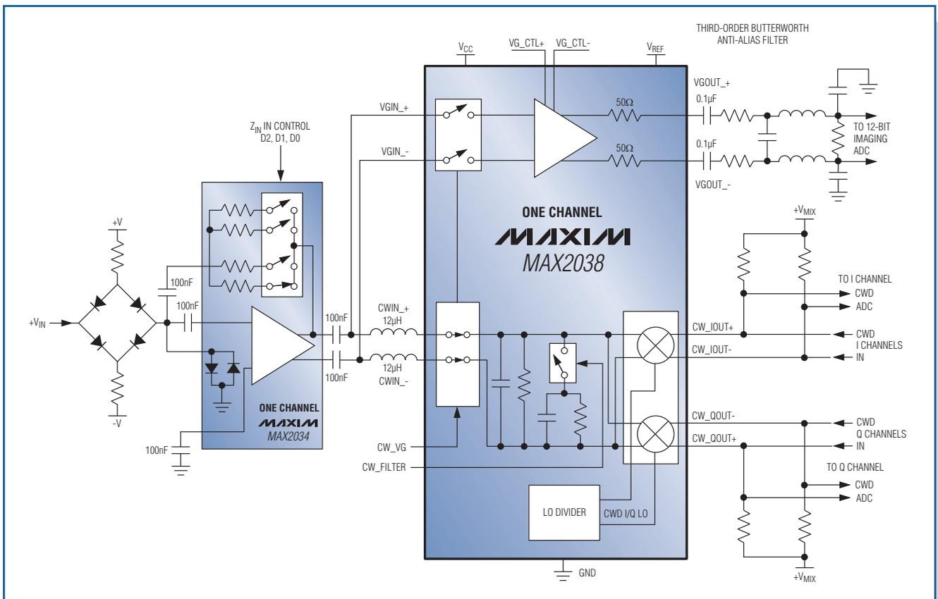
This simplified single-channel ultrasound receiver features the MAX2038 and MAX2034. The MAX2038 integrates eight VGA and CWD mixer I/Q beamformer channels onto a single chip, and the MAX2034 integrates four LNA channels onto a single chip. (See article on page 15.)
