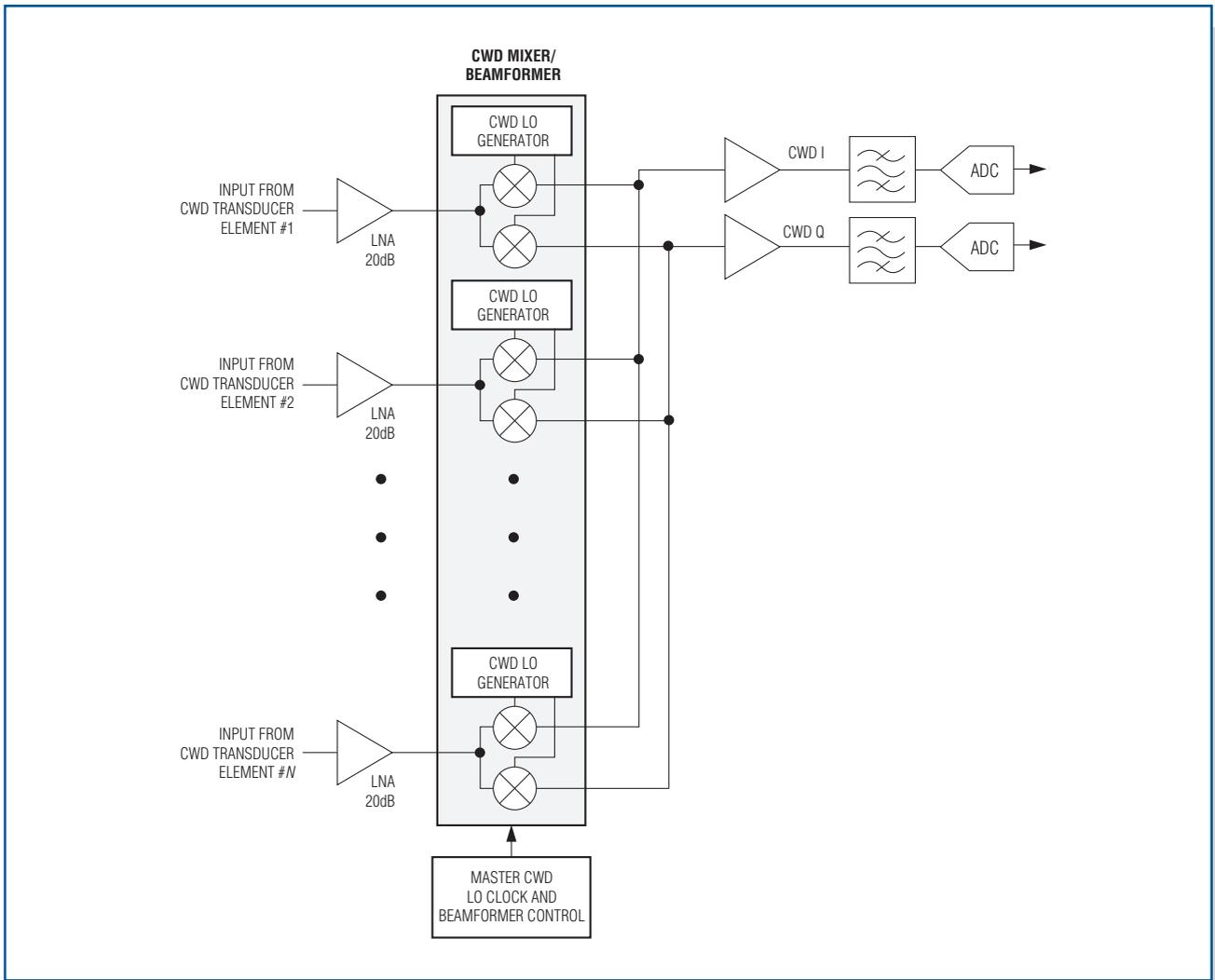
Figure 2. Low-power bipolar LNAs and a CWD mixer/beamformer can implement a simple, high-performance CWD receiver.
