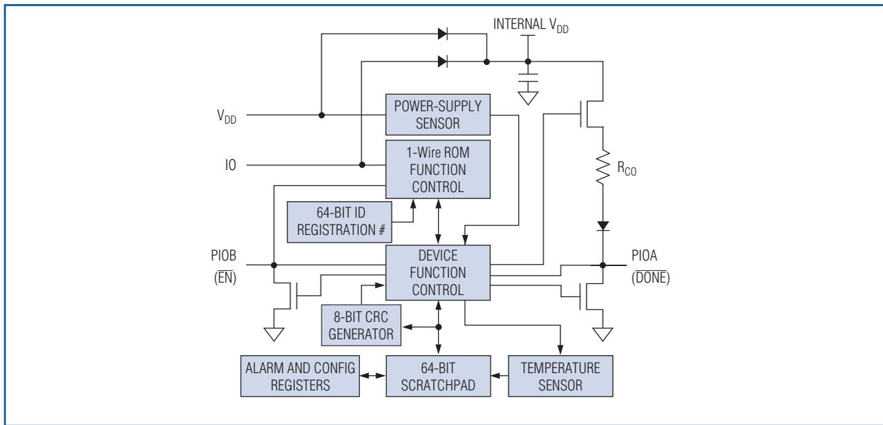
Figure 3. Able to run from either parasitically derived power or from an external supply, the DS28EA00 combines a temperature sensor, GPIO, alarm capabilities, and the 1-Wire interface in an 8-pin micro-small-outline package ( $\mu$ SOP).
