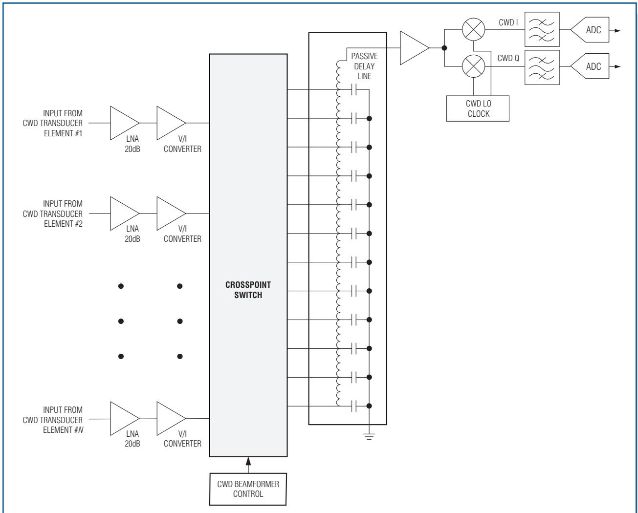
Figure 1. A simplified diagram of a CWD delay-line-based receiver.
