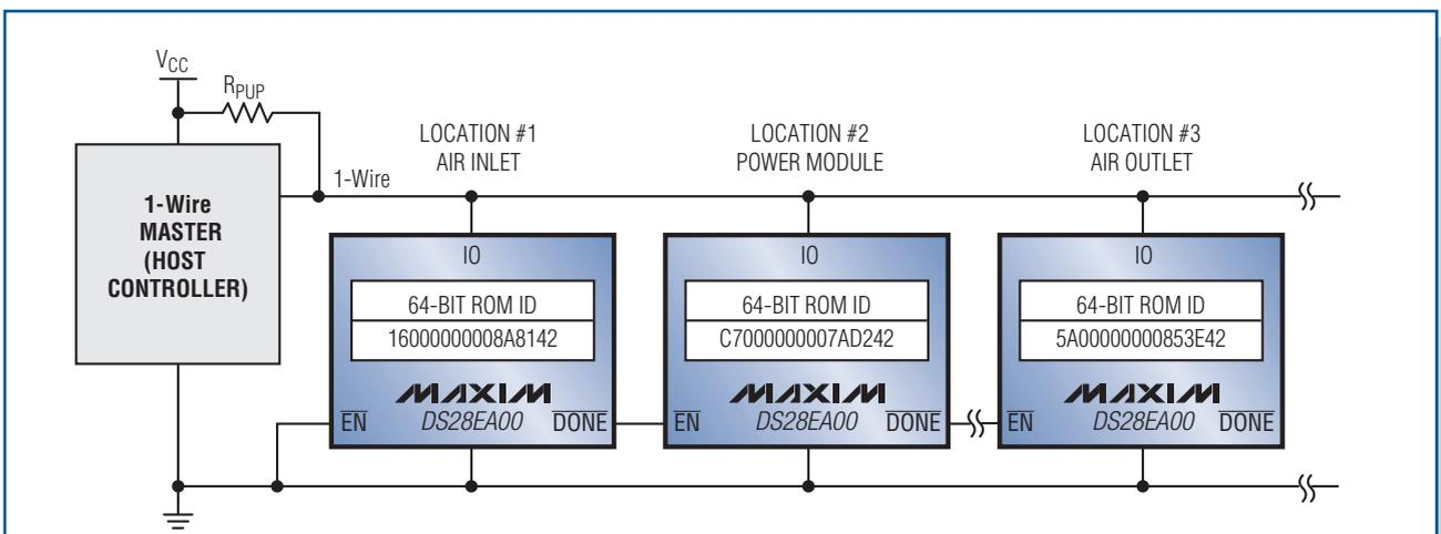
Figure 2. The DS28EA00 employs the chain-mode function in a typical 1-Wire network.
