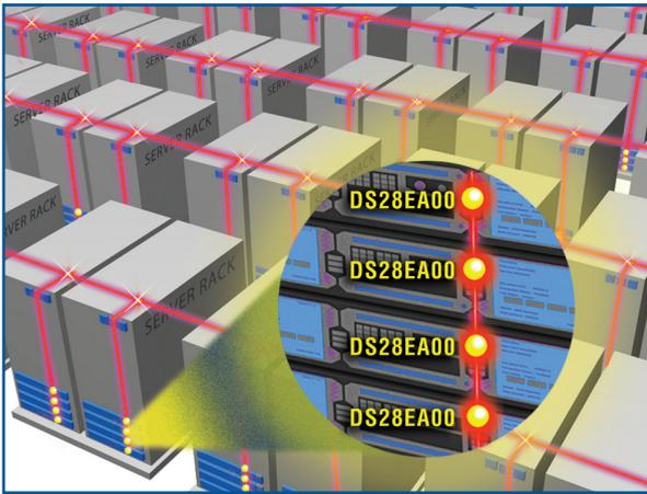
Figure 1. Energy management in a server farm can be improved by adding a network of 1-Wire digital temperature sensors, such as the DS28EA00, to monitor multiple locations for more efficient, controlled cooling.
