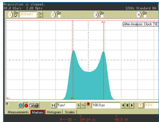
Figure 9. Measured TIE histogram.
