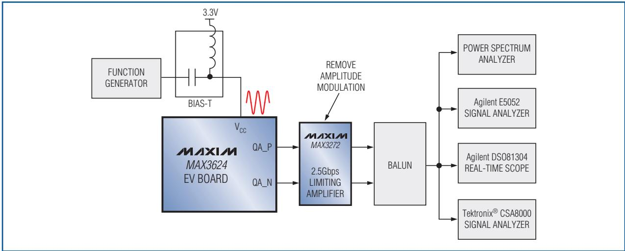
Figure 5. PSNR measurement setup.
