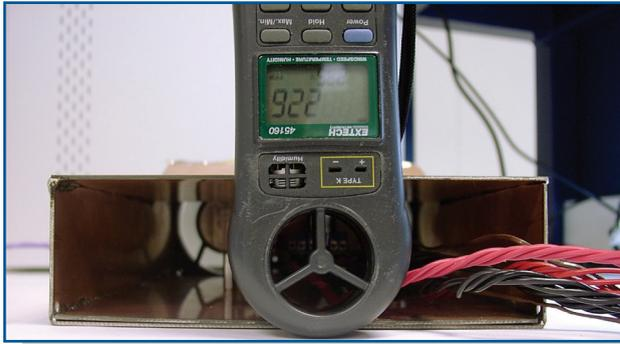
Figure 2. An airflow meter at the open end of the box measures the airflow to calibrate subsequent thermal measurements.
