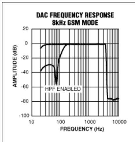
Figure 6. The frequency response of the GSM replay path has enabled GSM filters. At  $f_s = 8\text{kHz}$ , note the steep roll-off just before the Nyquist frequency (4kHz). The highpass filter (HPF) can be optionally
