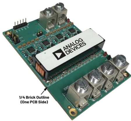
Figure 5. 48 V to 12 V regulated first stage. Components are placed on the top PCB side inside the 1/4-brick outline. Moving all ~1 mm components to the bottom: 1/8-brick.
