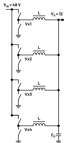
Figure 1. Four-phase buck converter with discrete inductors.
