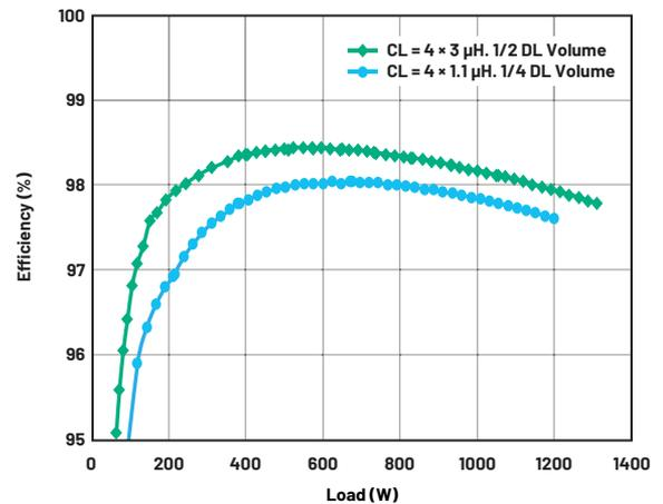
Figure 8. Efficiency vs. size trade-off for the proposed 48 V to 12 V solution with coupled inductors.
