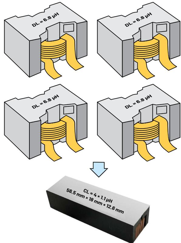
Figure 4. Four DL = 6.8  $\mu\text{H}$  inductors (top) are replaced with CL = 4  $\times$  1.1  $\mu\text{H}$  (bottom), achieving 4 $\times$  volume reduction.
