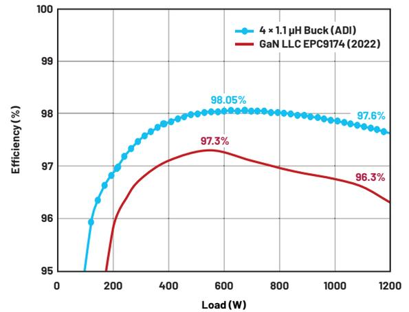
Figure 7. Efficiency comparison of the state-of-the-art 48 V to 12 V solutions in 1/8-brick form factor.
