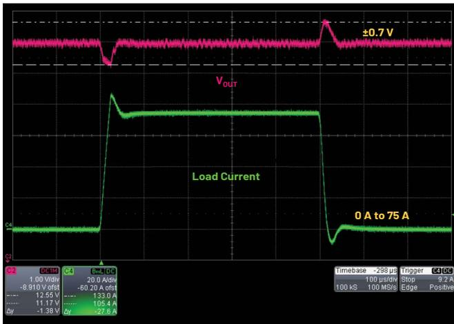
Figure 6. Transient at the  $V_0 = 12 \text{ V}$  output (CL =  $4 \times 1.1 \mu\text{H}$ ) for the 75 A load steps.
