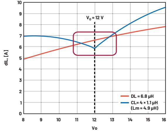
Figure 3. Current ripple for DL = 6.8  $\mu\text{H}$  and CL = 4  $\times$  1.1  $\mu\text{H}$  for  $V_{IN} = 48$  V and  $F_S = 200$  kHz as a function of  $V_o$ . The region of interest is highlighted.
