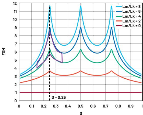
Figure 2. FOM for a 4-phase CL for some different  $L_m/L_k$  values as a function of the duty cycle  $D$ . The region of interest is highlighted.
