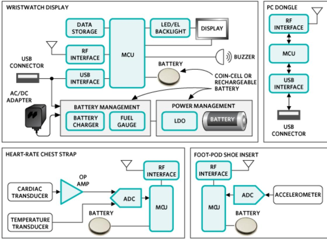
Figure 2. A typical data collection system for the heart-rate monitor consists of several subsystems. The wristwatch display/data storage unit (upper left), the wireless dongle to connect to the host computer (upper right), the heart-rate chest strap (lower left) and the shoe insert (lower right). Each of these subsystems requires a low-power wireless module.
