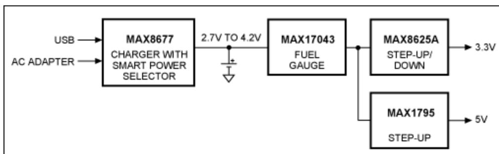
Figure 5. Power-supply example for a handheld spirometer using a single Li+ rechargeable battery.
