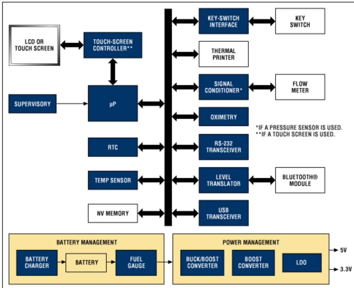
System block diagram of a desktop spirometer. For a list of Maxim's recommended solutions for spirometers, please visit: [www.maximintegrated.com/spirometer](http://www.maximintegrated.com/spirometer).
