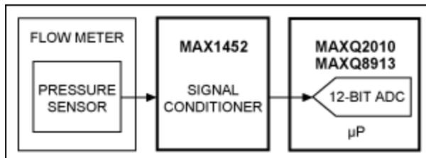
Figure 2. Typical front-end for a pressure sensor.
