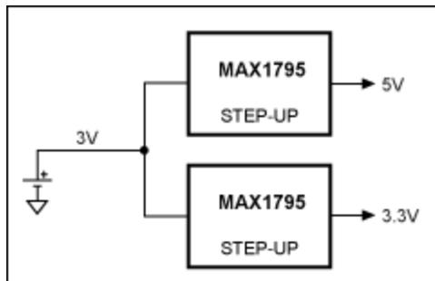
Figure 4. Power-supply example for a handheld spirometer using a coin-cell source.
