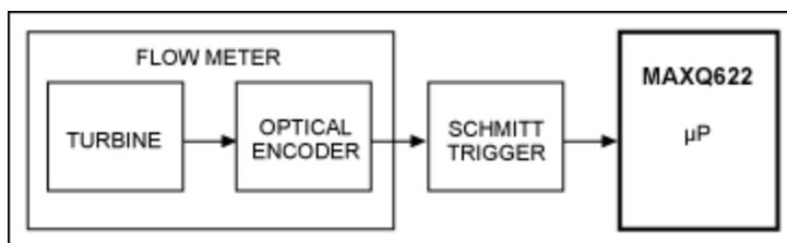
Figure 1. Typical front-end for a turbine transducer.
