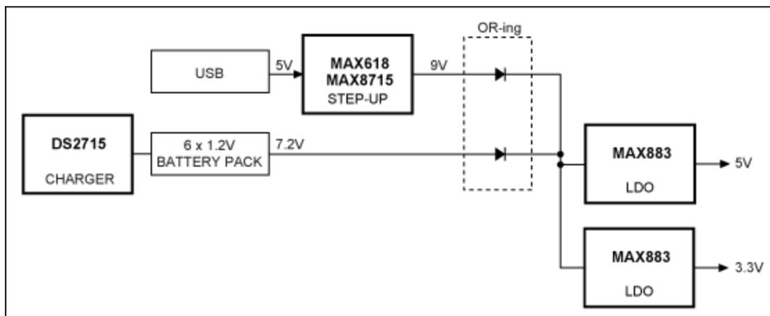
Figure 3. Power-supply example for a desktop spirometer.
