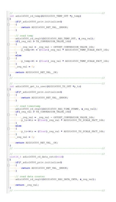
Figure 9: ADIS16500 read temperature, timestamp, data counter functions implementation
