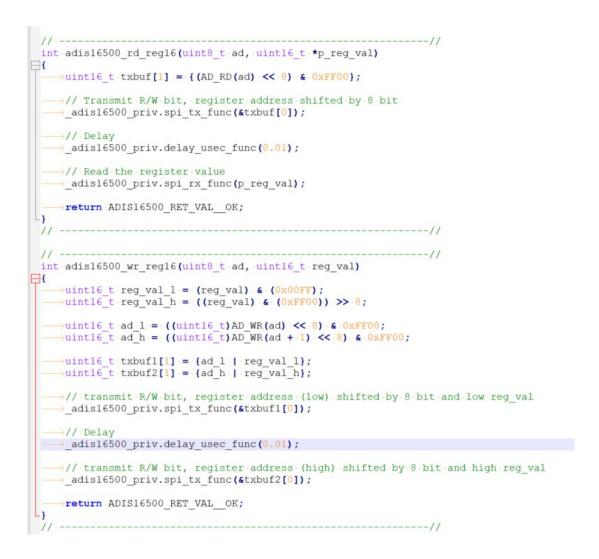
Figure 6: ADIS16500 read and write register functions implementation
