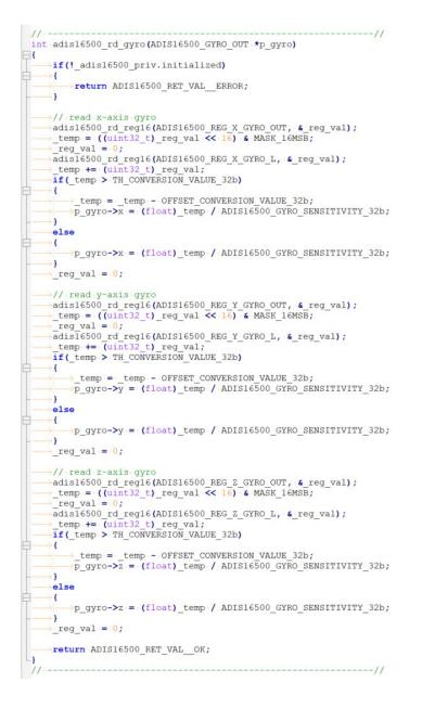
Figure 8: ADIS16500 read gyroscope function implementation
