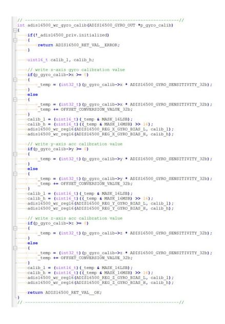
Figure 12: ADIS16500 write gyroscope calibration function implementation
