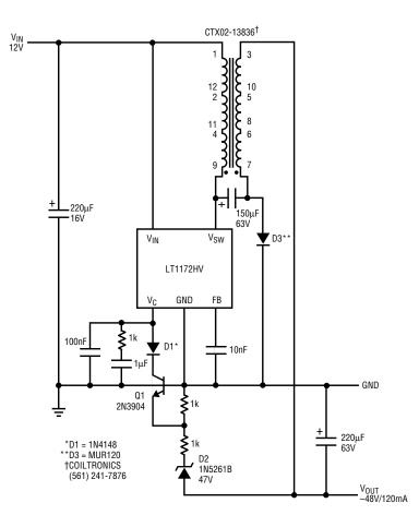
Figure 1. 12V to -48V features good efficiency over a wide range of loads.
