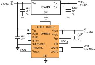
The ultrathin LTM4632 provides a complete high performance regulator solution for all three rails required in DDR/QDR RAM applications. Its wide operating range, features and compact solution size make it highly flexible and robust, and capable of fitting into the tightest spaces on the topside and backside of a PCB.
