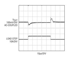
Figure 5. VTT load step, -3A to 3A (Figure 2 design)
