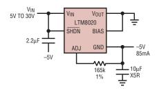
Figure 2. A simple reconfiguration of the  $\mu$ Module generates a negative output
