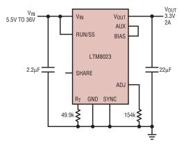
Figure 5. The LTM8023 produces 3.3V at 2A with the same footprint and components required for the LTM8022 producing 1A.
