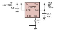
Figure 1. Generate 3.3V at 200mA with the LTM8020, two caps and a resistor
