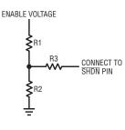
Figure 7. Programming the enable voltage by using external resistors
