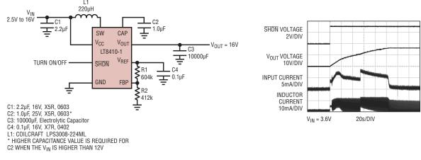
Figure 6. Capacitor charger with the LT8410-1 and charging waveforms
