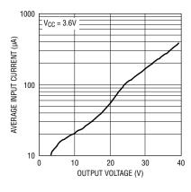
Figure 4. Average input current in regulation with no load
