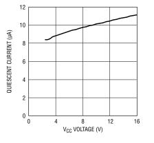
Figure 3. Quiescent current vs V<sub>CC</sub> voltage—not switching
