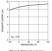
Figure 2. Quiescent current vs temperature—not switching
