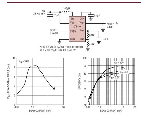
Figure 5. General purpose bias with wide input voltage and low output voltage ripple
