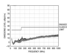
Figure 4. The LTM8032 emissions for 20W out,  $36V_{IN}$
