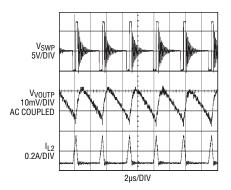
Figure 4. Switching waveforms at 10mA load for the boost application shown in Figure 2
