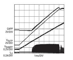
Figure 8. V<sub>OUTP</sub> soft-start ramping from ground
