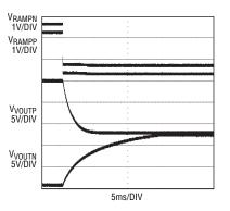
Figure 9. Power-down discharge waveforms
