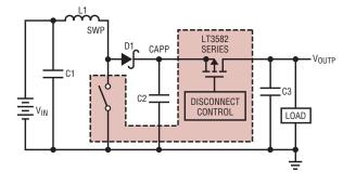
Figure 7. Output disconnect PMOS
