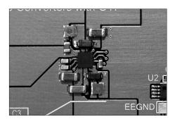
Figure 1. Dual output supplies in a small board footprint
