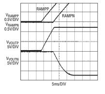
Figure 6. Power-Up Sequencing  $(V_{OUTP} \text{ followed by } V_{OUTN})$
