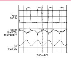
Figure 5. Switching waveforms at 100mA load for the boost application shown in Figure 2
