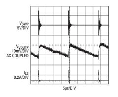
Figure 3. Switching waveforms at 1mA load for the boost application shown in Figure 2
