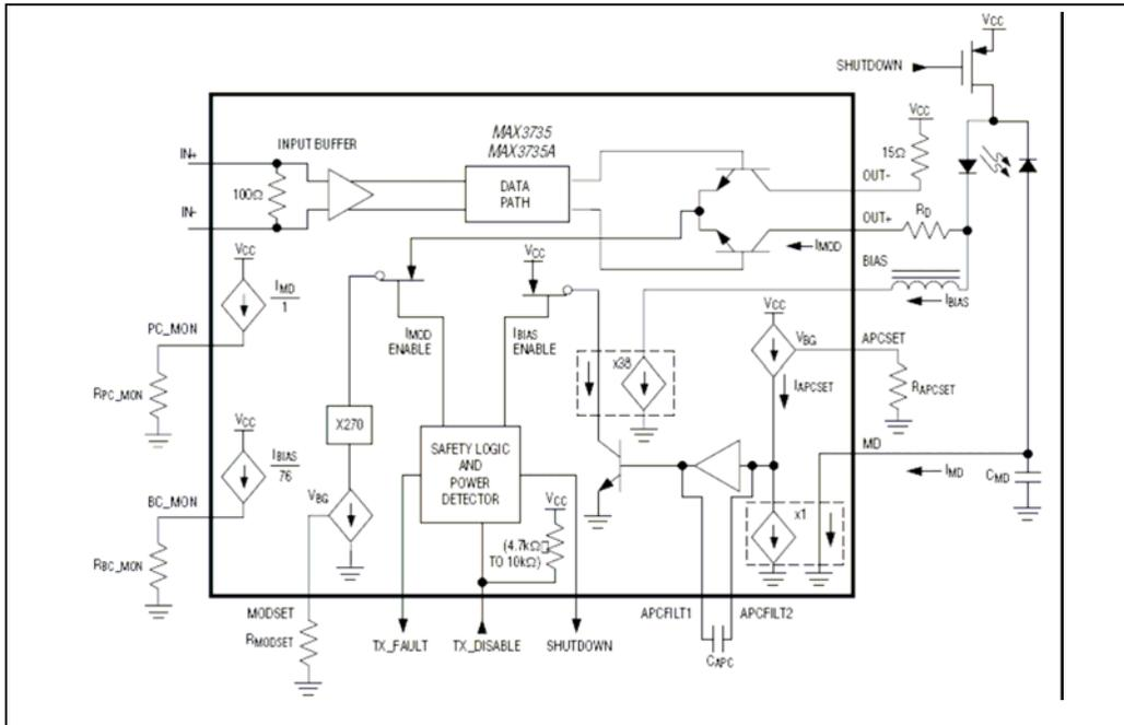
Figure 1: Conventional Monitor Block Diagram
