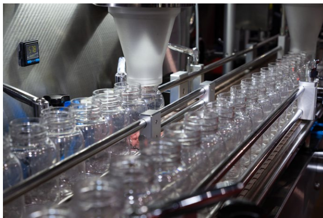
Figure 9. Damage and defects can be detected before bottling where it often is not practical to set up a large vision system (which is more often used after the bottles are filled and packaged). This is especially helpful when the bottles are visually difficult to distinguish from one another.
