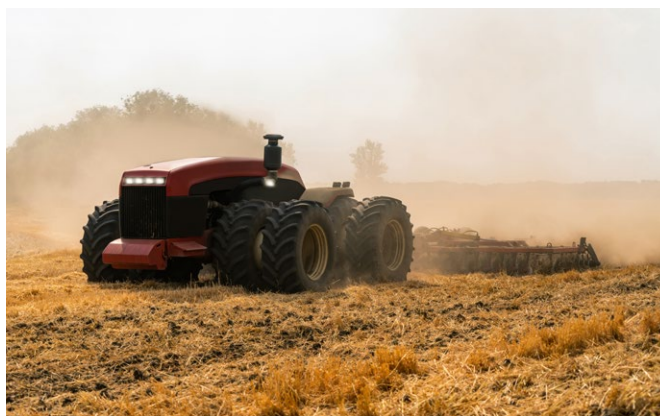
Figure 8. The plowing of a field with subsequent real-time terrain mapping—insensitive to lighting conditions due to the nature of LIDAR.
