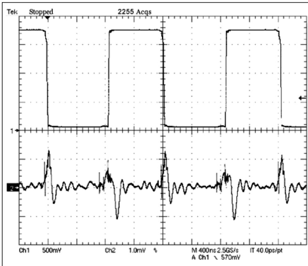
Figure 7. The MAX9509's output (bottom trace) is measured vs. time, taken with respect to a 1V<sub>P-P</sub> video signal. The spikes are 1.4mV<sub>P-P</sub>. The top trace is the voltage on the top plate of the charge pump's flying capacitor.
