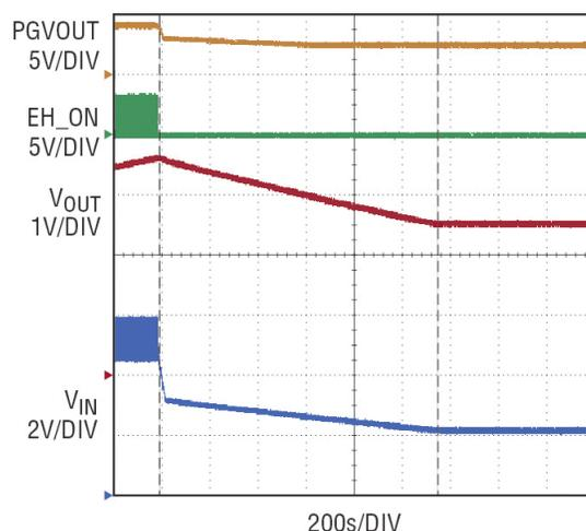
**Figure 5. Output supercapacitor discharging when the vibration source is switched off**
