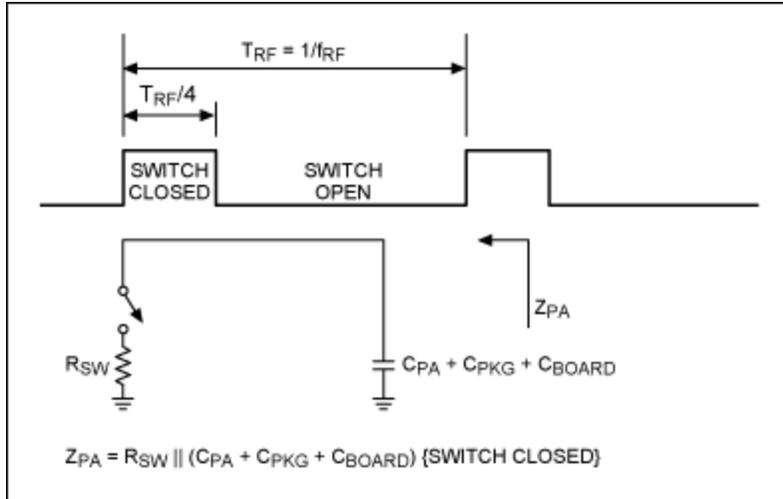
Figure 3. Simplified model of a switching-mode amplifier.
