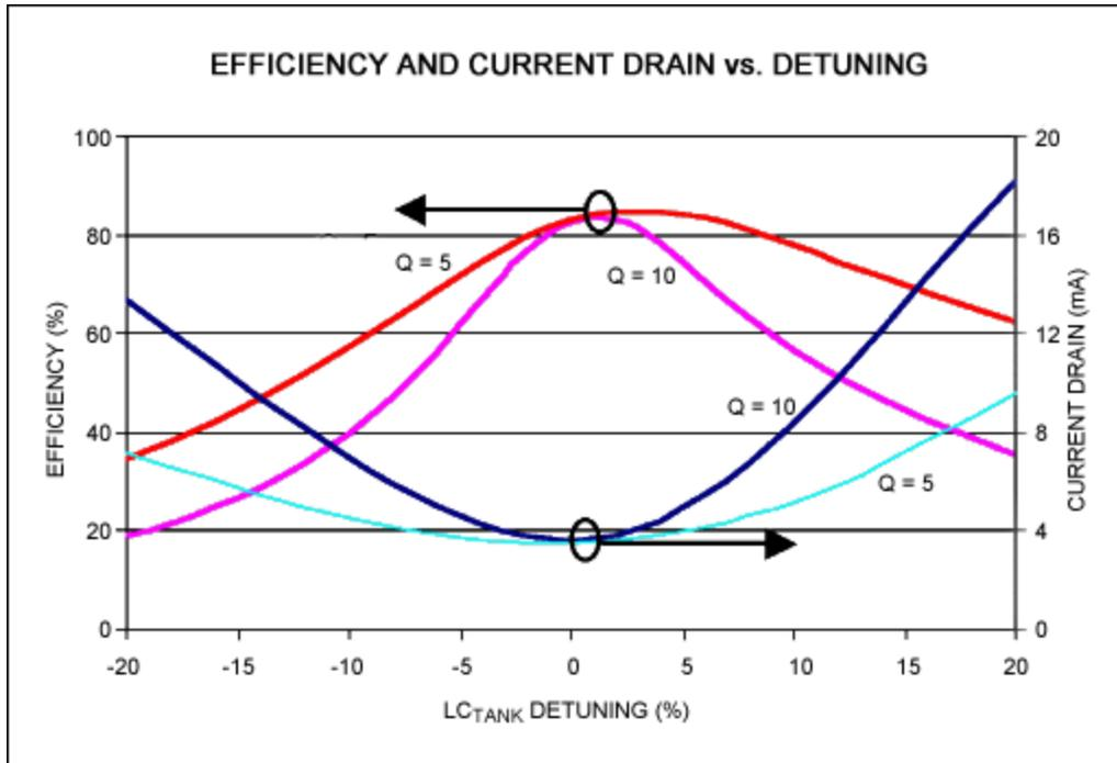
Figure 7. Ideal switching-mode amplifier performance vs. detuning.
