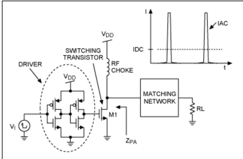
Figure 2. Schematic of a switching-mode amplifier.
