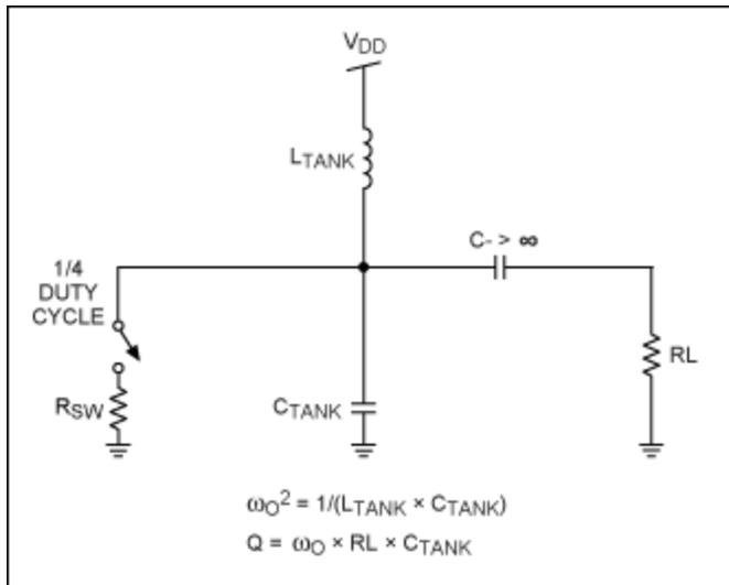
Figure 5. Simulation schematic for an ideal switching-mode amplifier.
