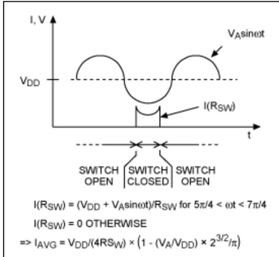
Figure 4. Switching-mode amplifier waveform.
