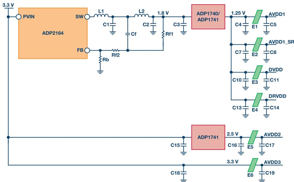
Figure 2: Simplified PDN for the AD9680 evaluation board.
