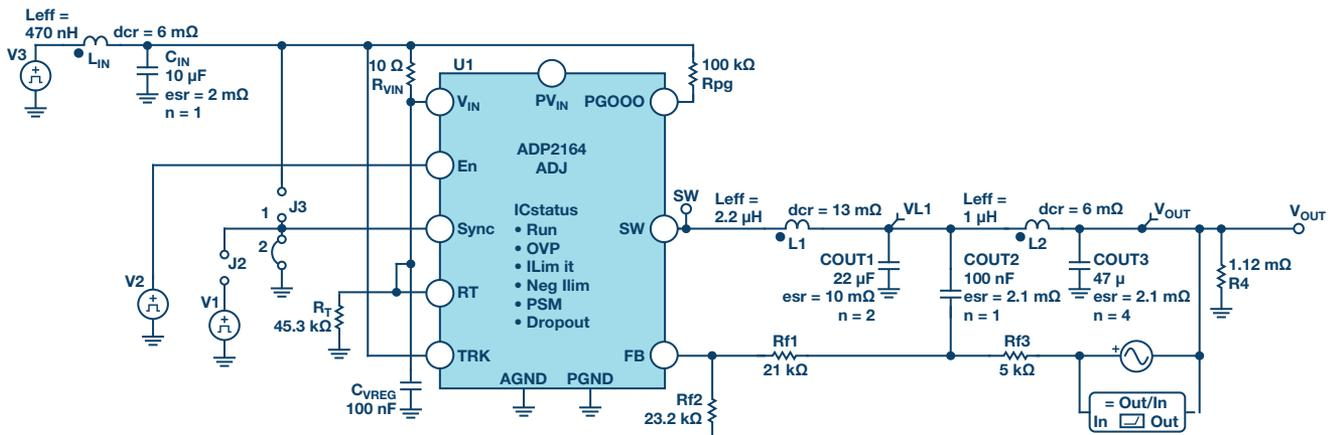
Figure 8. ADIsimPE schematic of ADP2164 driving the 1.25 V domains.
