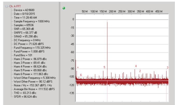
Figure 4. Single-tone FFT at 170 MHz input, with PDN #3.
