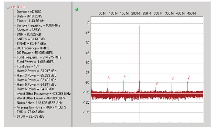
Figure 5. Single-tone FFT at 785 MHz input, with PDN #3.
