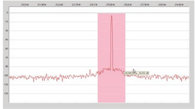
Figure 7. 1.2 MHz sideband switching spur at 785 MHz input. Spur level = -94 dBFS.
