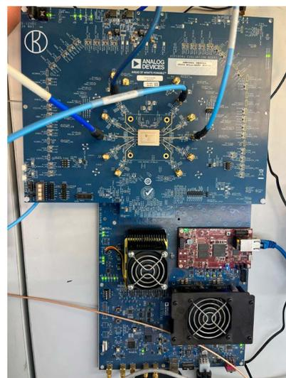
Figure 14. ADS10-V1EBZ (motherboard) and ADRV904X-MB/PCBZ evaluation board.
