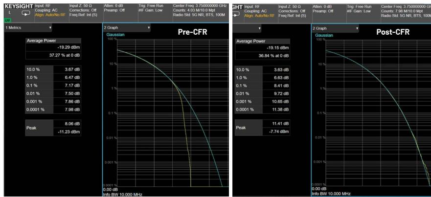
Figure 10. 5G NR signal before and after applying CFR.
