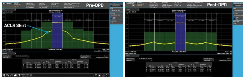
Figure 12. Power spectral density showing improvement in ACLR post-DPD.
