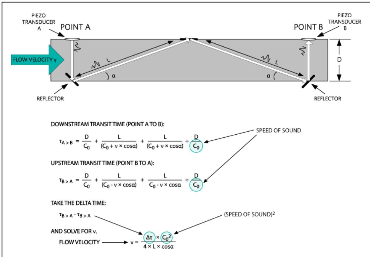
Figure 1. Example time-of-flight difference calculation.
