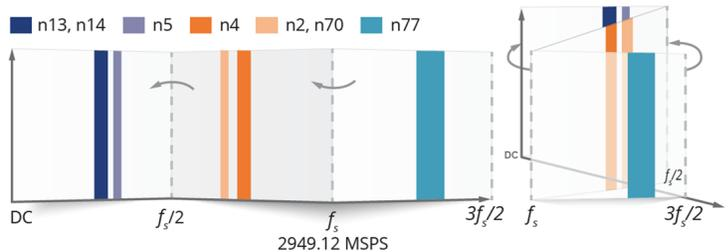
This illustrates spectrum folding back onto the first and second Nyquist zone creating aliases. Using a common sample rate, 2949.12, band n77 (C-Band) will alias with bands n2, n4, n5, n13, n14 and n70, increasing filter requirements, adding weight, and cost.
