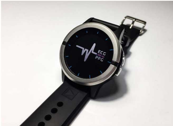
Figure 1. The VSM study watch development platform created by Analog Devices.
