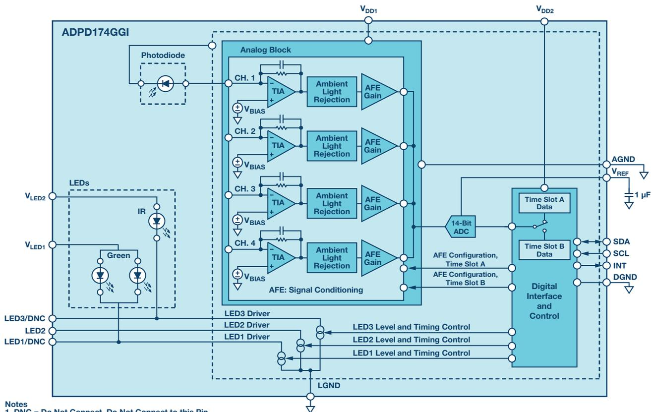
Figure 3. Block diagram of the ADPD174 optical subsystem.
