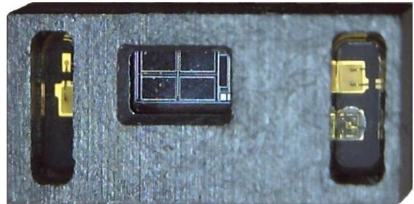
Figure 1. ADPD174, optical 6.5 mm  $\times$  2.8 mm system in a single package.
