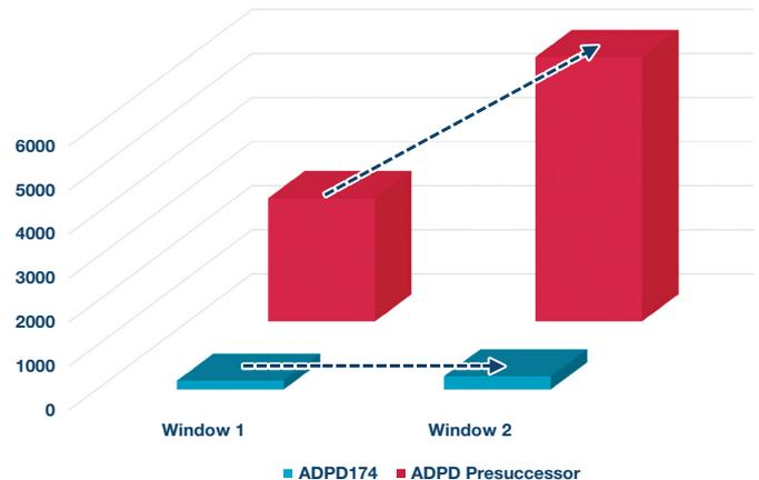
Figure 5. ADPD174 ILP impact vs. its predecessor.
