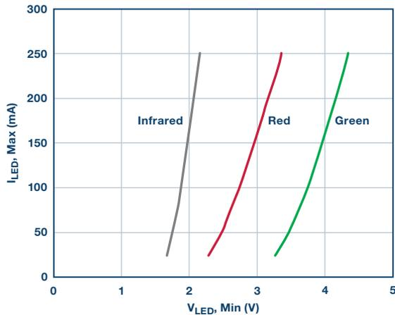
Figure 2. Required LED forward voltage vs. LED current.
