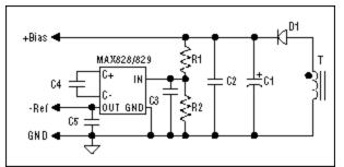
Figure 2. -Ref circuit employing the MAX828/MAX829 charge-pump IC.
