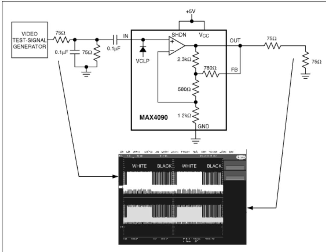
Figure 1b. DC-coupled output connection.
