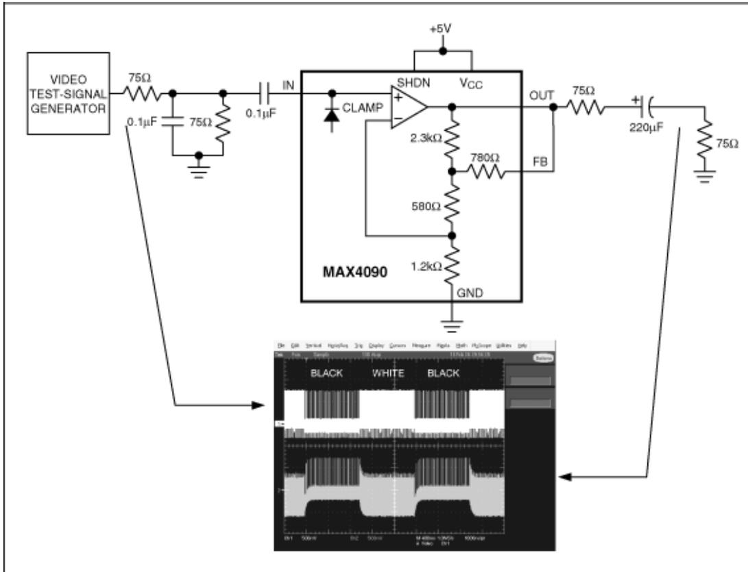
Figure 1a. AC-coupled output connection.
