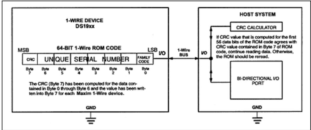
Figure 1. iButton system configuration using 1-Wire CRC.
