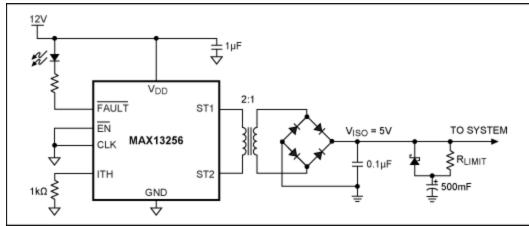
Figure 2. Sample MAX13256 supercap charging circuit.
