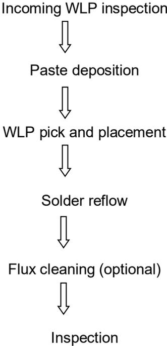
Both solders paste or flux printing and dipping approaches provide acceptable assembly quality and reliability. Maxim Integrated WLP meets Joint Electron Device Engineering Council (JEDEC) level 1 moisture sensitivity classification. No baking is needed before assembly.
