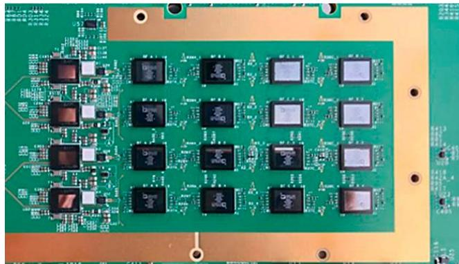
Figure 2. The component side of AiB256 (16 beamformers and four mmWave up/downconverters).
