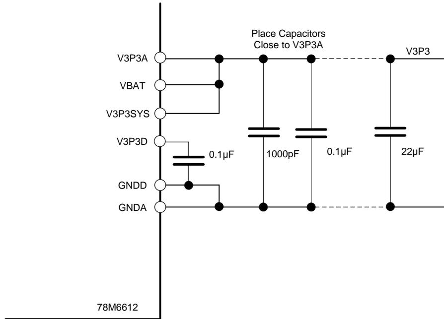
**Figure 2: Power Supply Decoupling**
