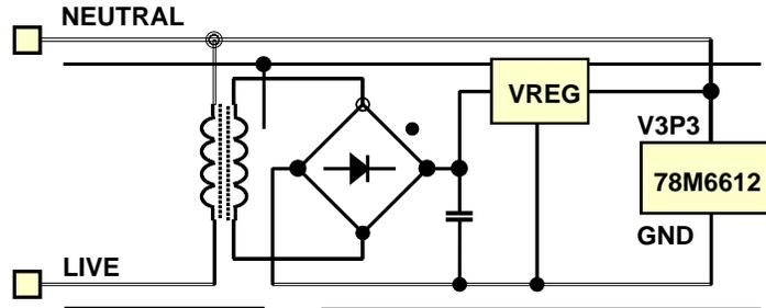
Figure 17: No High-Voltage Components for Higher Power Applications
