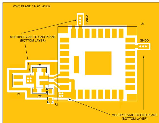
Figure 24: Example of Layout of Crystal Oscillator with Pull-up Resistor
