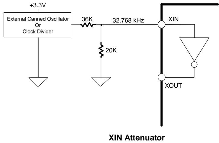
Figure 25: 78M6612 with External Canned Oscillator
