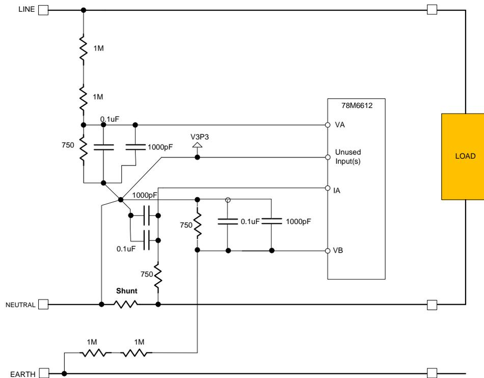
**Figure 1: Basic Connection Diagram on Shunt-Based Systems**
