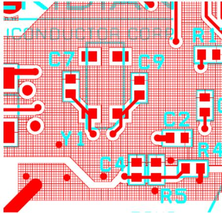
Figure 20: Crystal Y1 and Capacitors C7/C9
