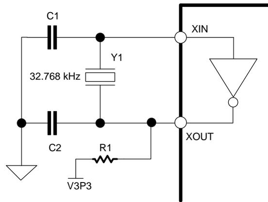
Figure 23: Crystal Oscillator with Pull-up to Reduce Startup Time
