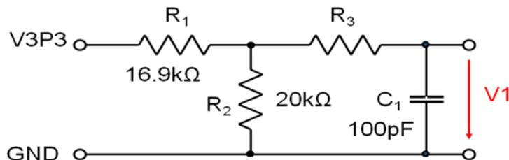
Figure 10: Voltage Divider
