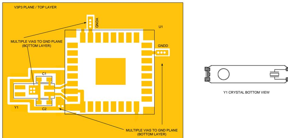
Figure 22: Crystal Oscillator Components on the Same Side
