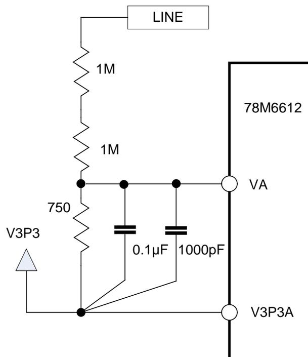
**Figure 3: Input Voltage Divider and Filtering**
