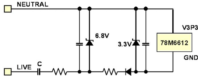
Figure 16: Simple Circuit Design for Low-Power Applications
