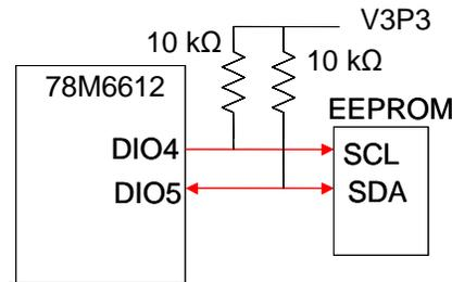
**Figure 13: I<sup>2</sup>C EEPROM Connection**
