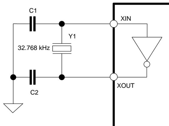
**Figure 19: 78M6612 Crystal Oscillator Connection**
