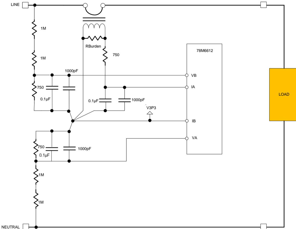
**Figure 6: Basic Connection Diagram of a CT-Based System**
