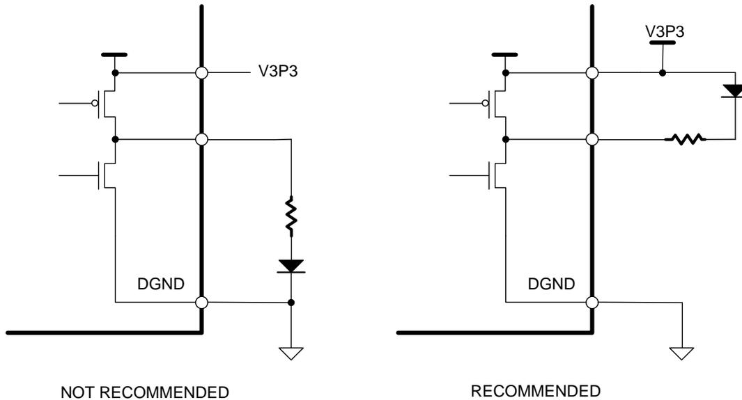
**Figure 12: Connecting an External Load to a Digital Output**
