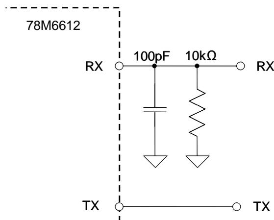
Figure 15: Connections for the RX Pin
