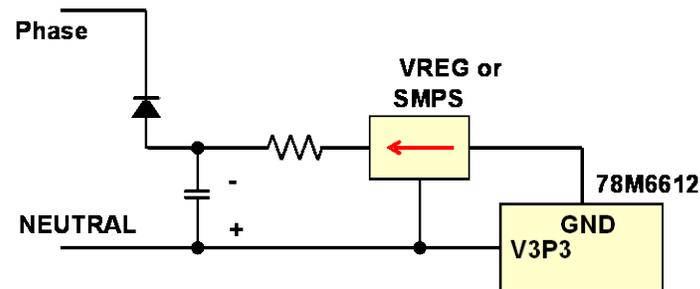
Figure 18: High Efficiency for Higher Power Applications
