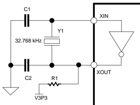
Figure 22: Crystal Oscillator with Pull-up to Reduce Startup Time
