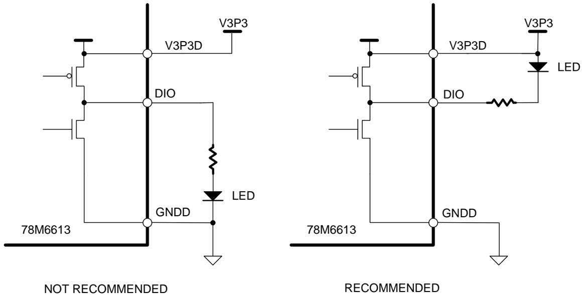
Figure 11: Connecting an External Load to a Digital Output
