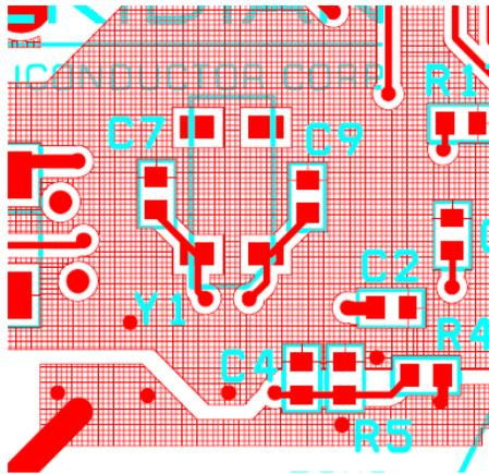
Figure 19: Crystal Y1 and Capacitors C7/C9
