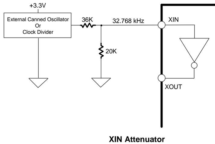
Figure 24: 78M6613 with External Canned Oscillator
