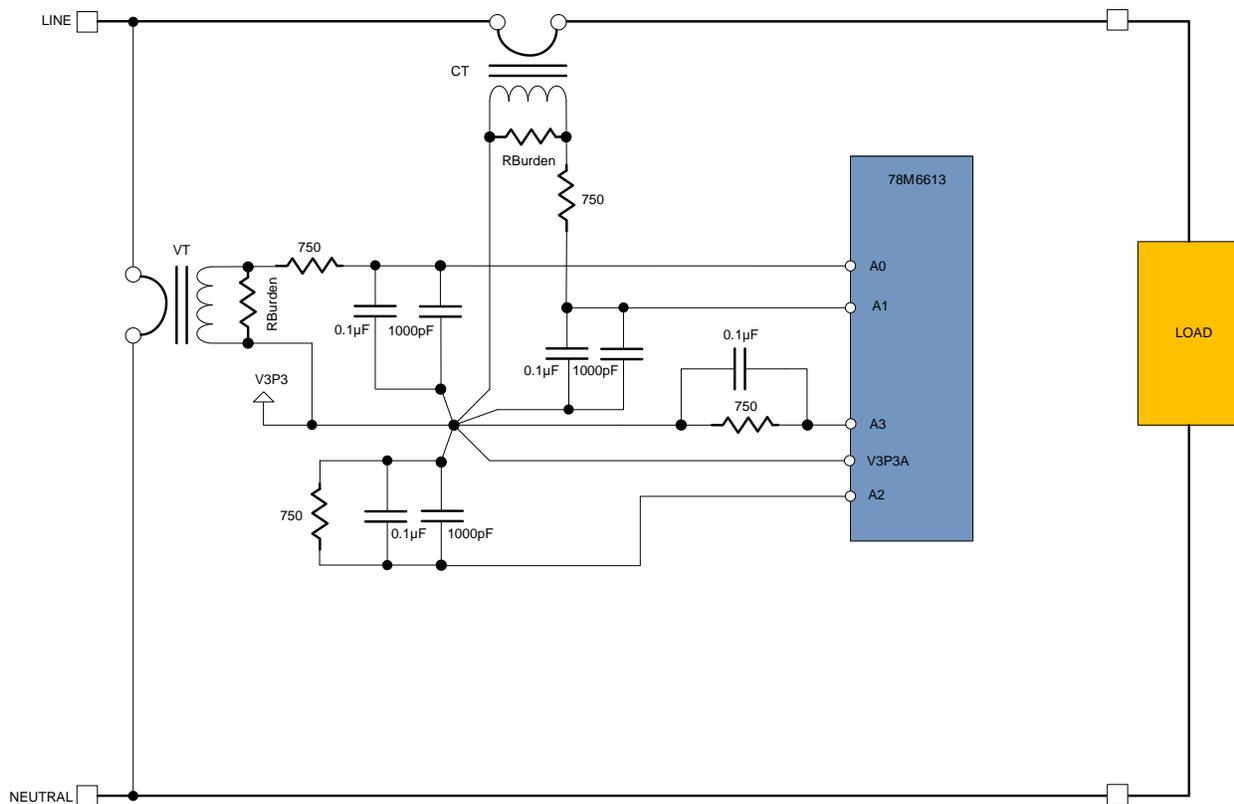
Figure 7: Basic Connection Diagram of a CT and VT Based System
