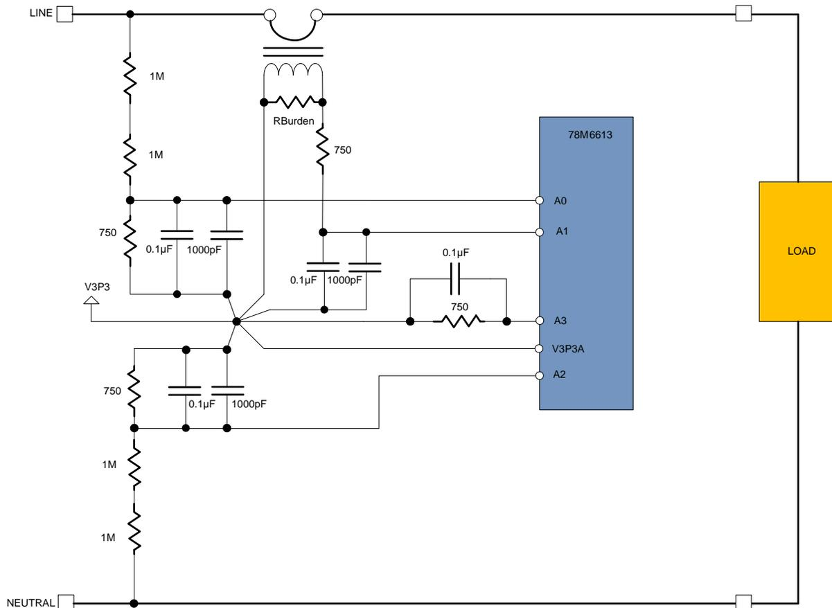
**Figure 6: Basic Connection Diagram of a CT-Based System**
