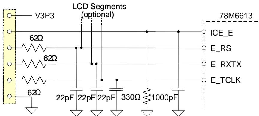
Figure 10: ICE Pin Used to Drive LCD Segments
