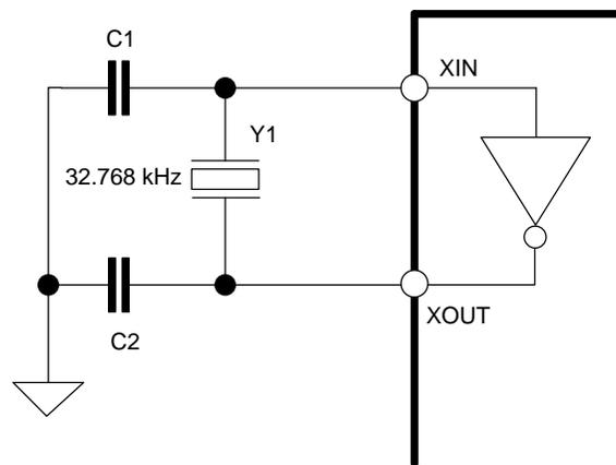
**Figure 18: 78M6613 Crystal Oscillator Connection**
