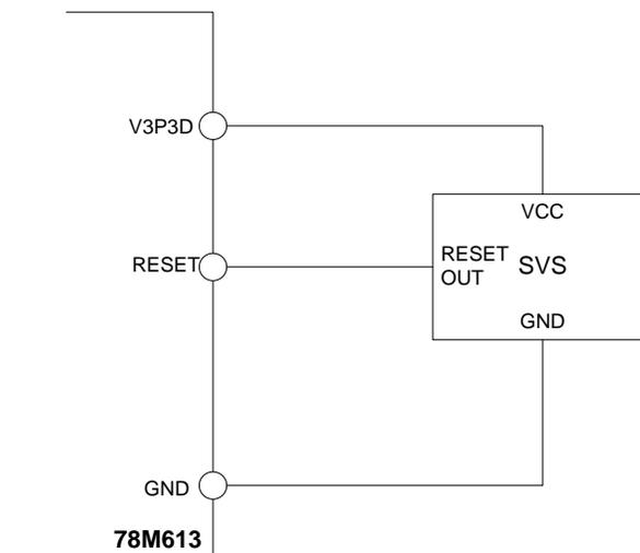
Figure 9: Reset Generator Connection
