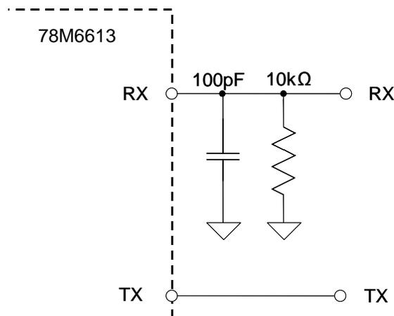
Figure 14: Connections for the RX Pin
