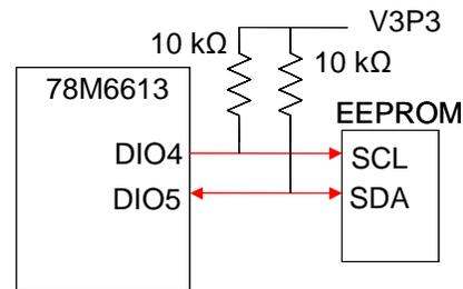
Figure 12: I<sup>2</sup>C EEPROM Connection
