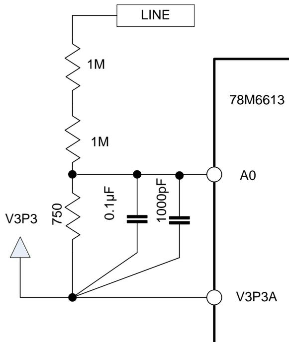
**Figure 3: Input Voltage Divider and Filtering**
