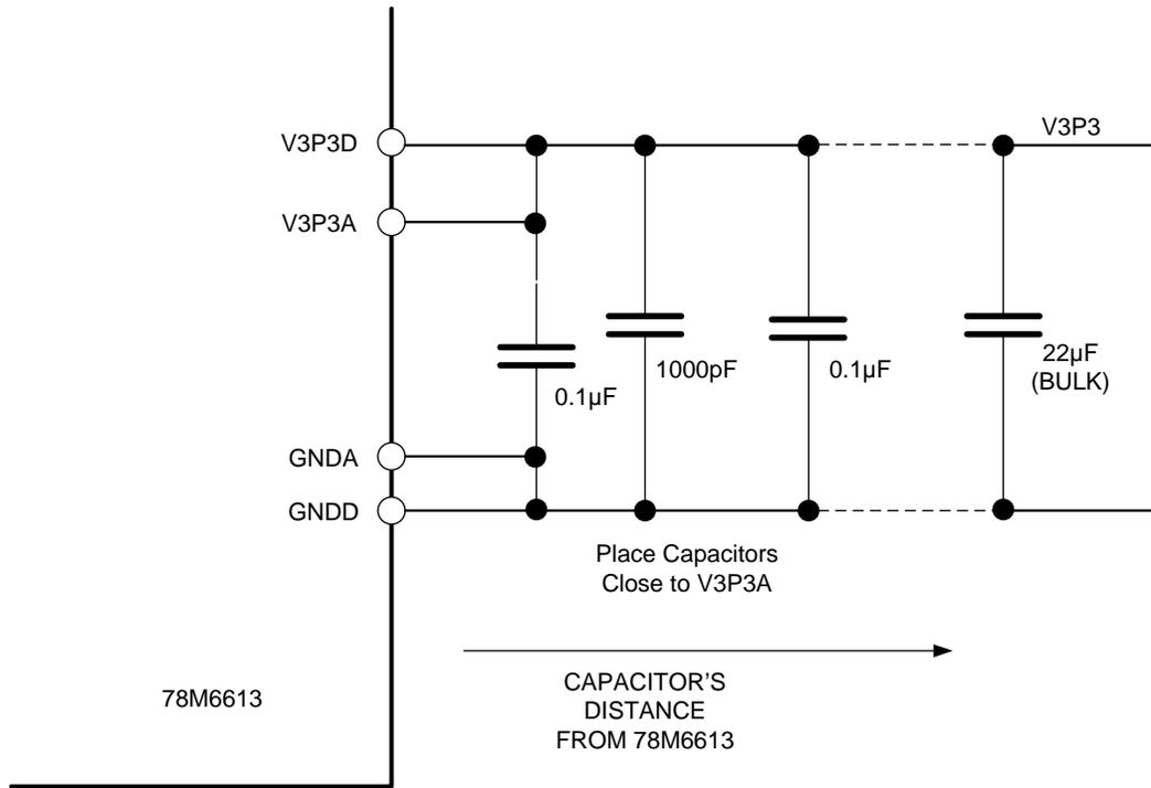
**Figure 2: Power Supply Decoupling**
