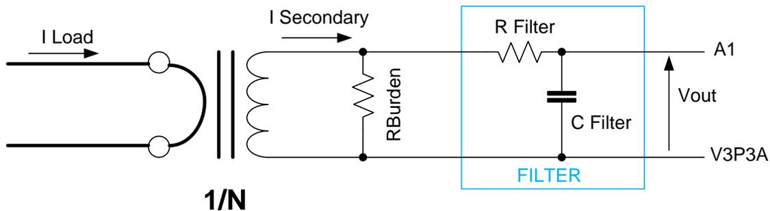
Figure 5: Current Transformer (CT) Basic Connections
