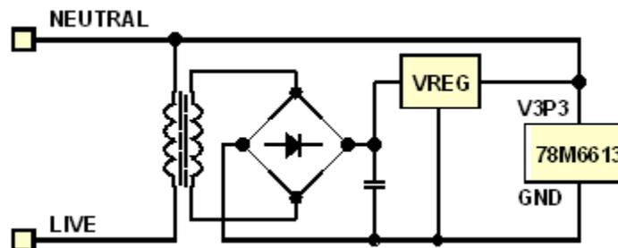
Figure 16: No High-Voltage Components for Higher Power Applications
