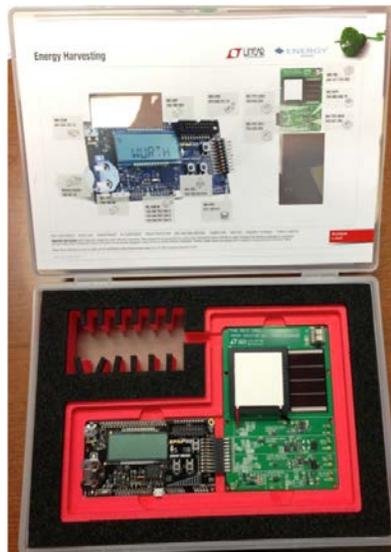
Figure 1. DC2080A Connected to an Energy Micro Starter Kit in the “To Go” Design Kit for Energy Harvesting
