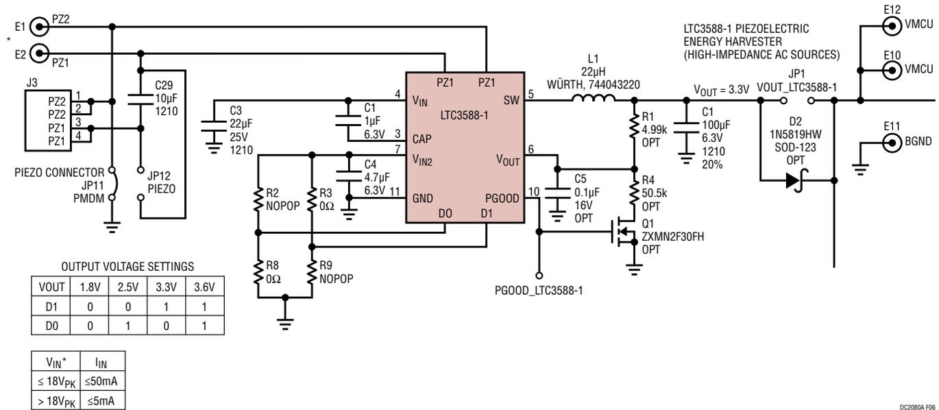
Figure 6. Detailed Schematic of LTC3588-1 Piezoelectric Energy Harvesting Power Supply
