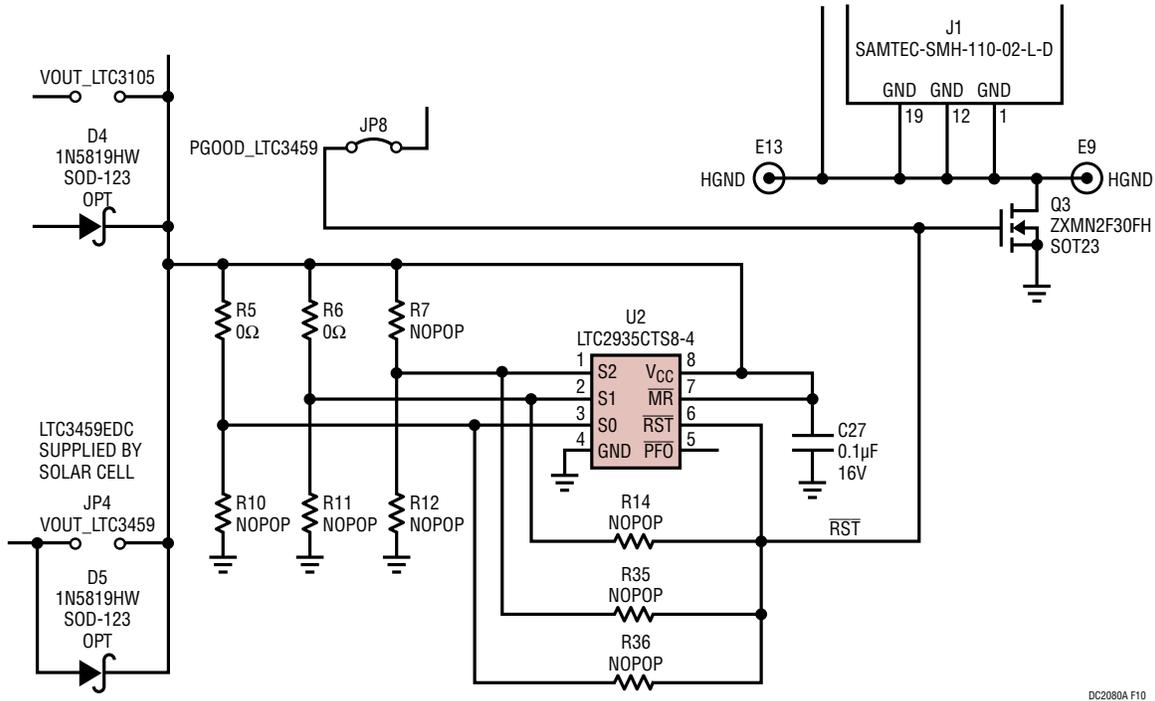
Figure 10. Detailed Schematic of PGOOD\_LTC3459 Circuit Using LTC2935-2
