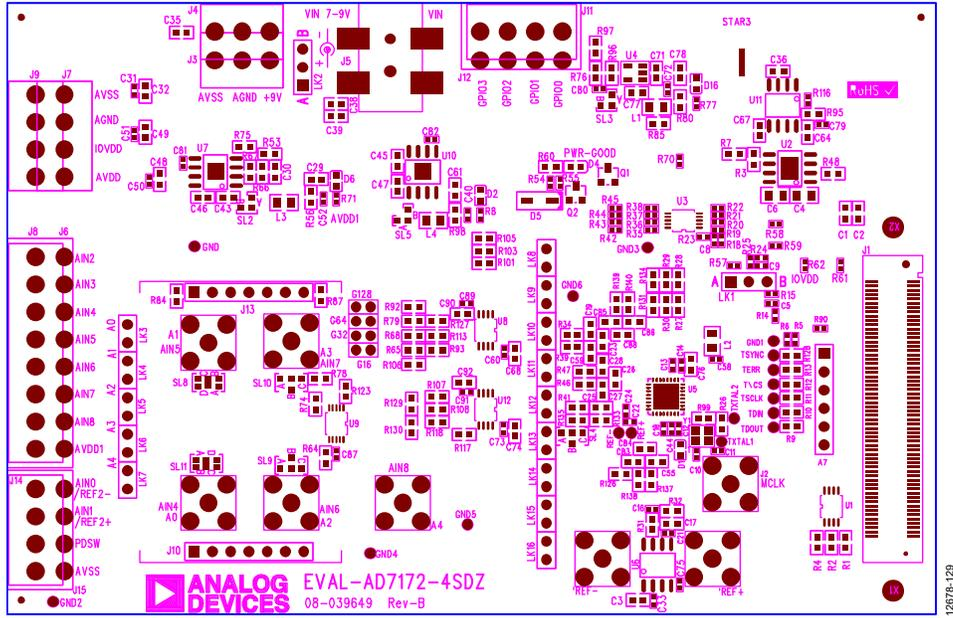
Figure 29. Top Printed Circuit Board (PCB) Silkscreen
