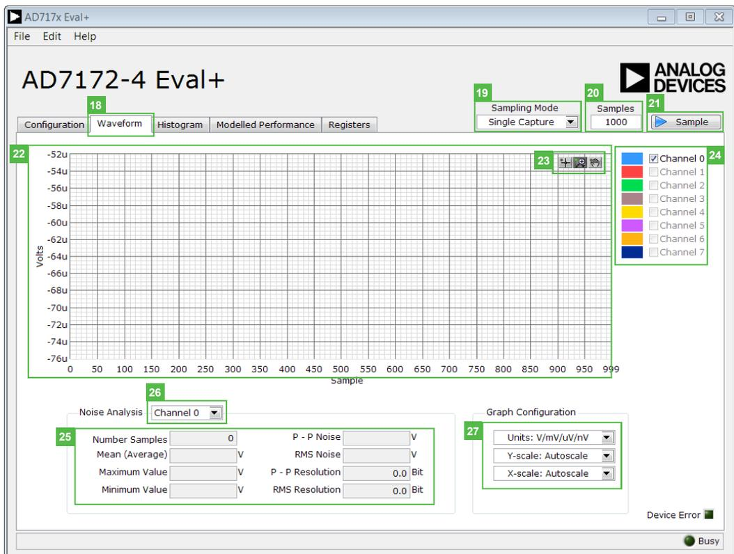
Figure 17. **Waveform** Tab of the [AD7172-4](#) Evaluation Software
