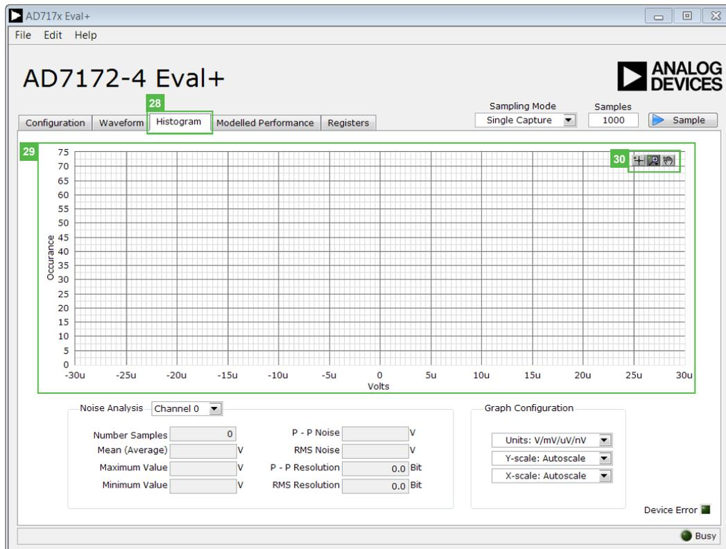
Figure 18. Histogram Tab of the AD7172-4 Evaluation Software
