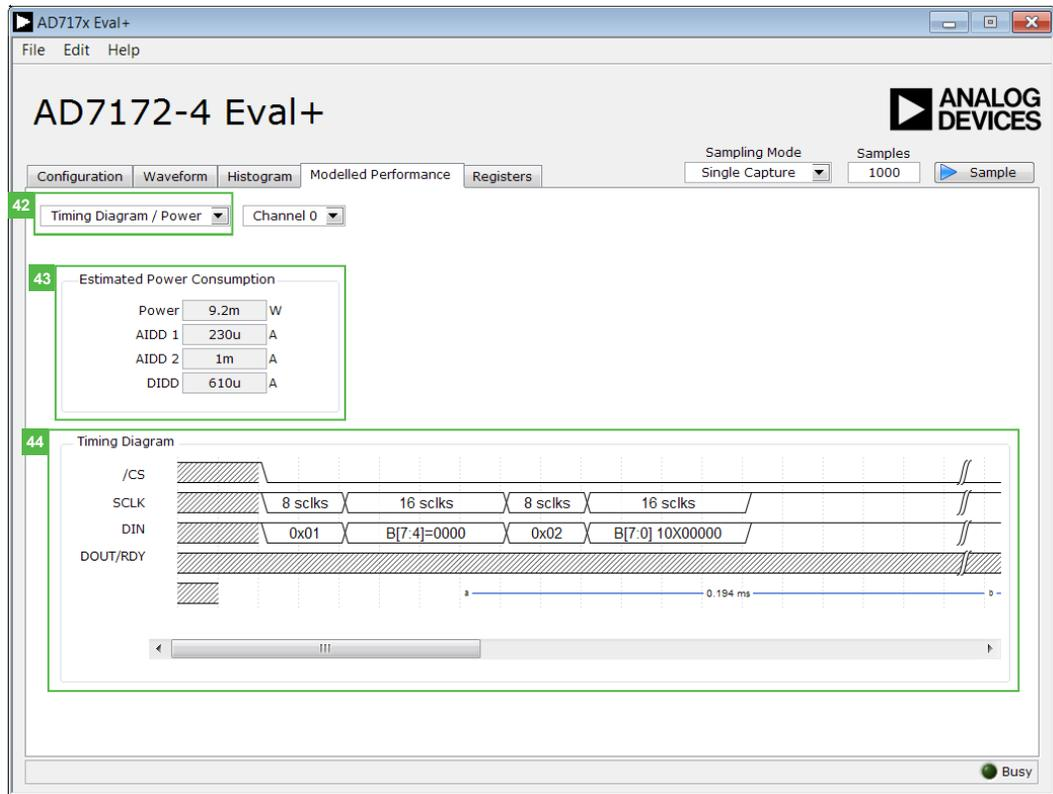
Figure 21. Timing Diagram/Power of the AD7172-4 Evaluation Software
