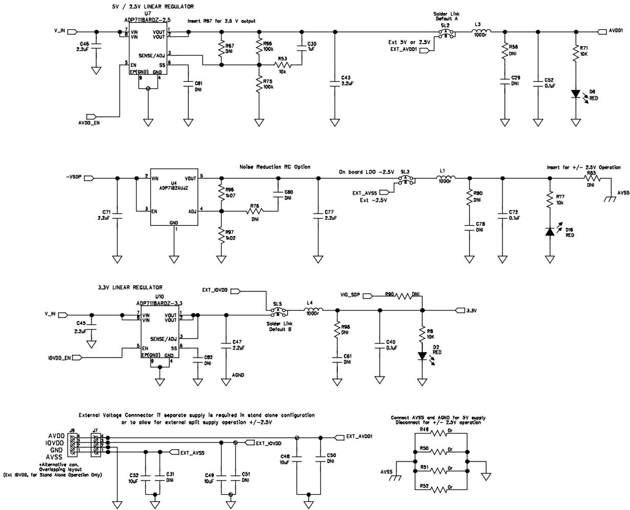
Figure 27. Regulator Schematic
